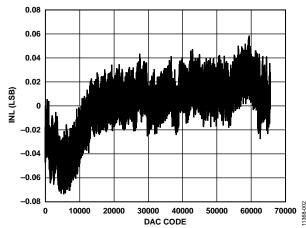
Figure 2. Integral Nonlinearity vs. DAC Code
