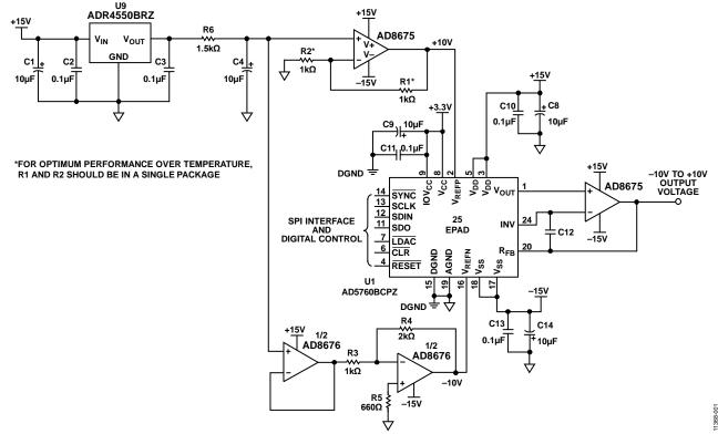
Figure 1. 16-Bit Accurate, ±10 V Voltage Source (Simplified Schematic: All Connections and Decoupling Not Shown)
