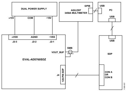
Figure 7. Functional Block Diagram of Test Setup
