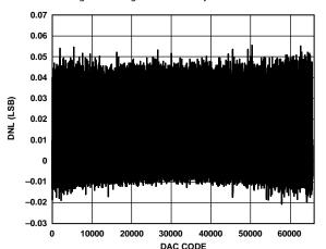
Figure 3. Differential Nonlinearity vs. DAC Code
