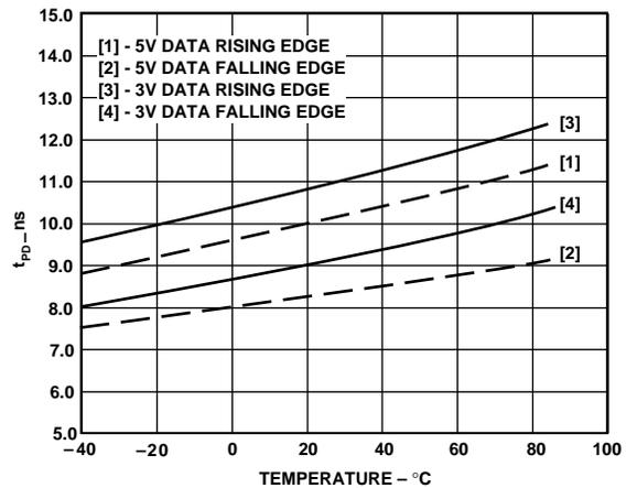
Figure 15.  $t_{PD}$  vs. Temperature 3 V/5 V
