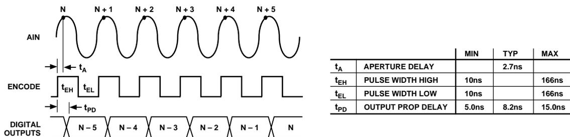
Figure 2. Timing Diagram
