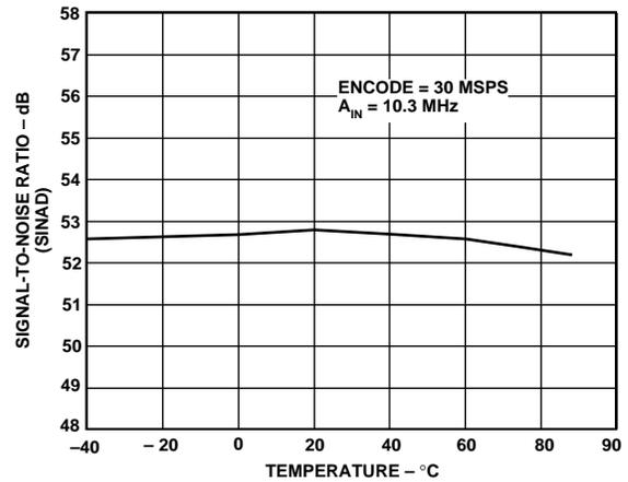
Figure 7. SNR vs. Temperature
