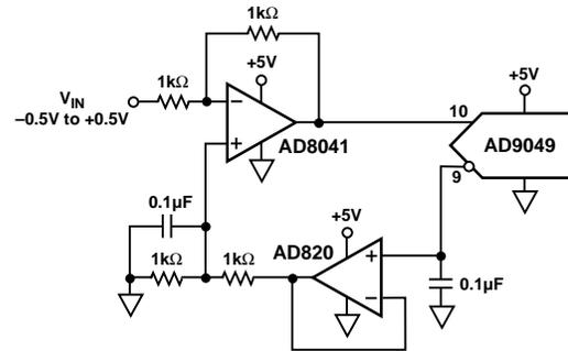
Figure 16. Single Supply, Single Ended, DC Coupled AD9049
