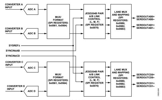
Figure 60. Transmit Link Simplified Block Diagram with Full Bandwidth Mode
