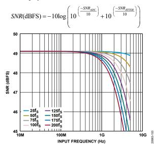
Figure 53. Estimated SNR Degradation vs. Analog Input Frequency over RMS Jitter
