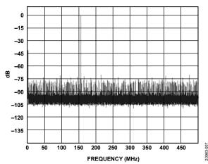
Figure 7. Single-Tone FFT with  $f_{\rm IN}$  = 155 MHz, SNRFS = 49.1 dBFS, SFDR = 71 dBFS, SINAD = 49.1 dBFS
