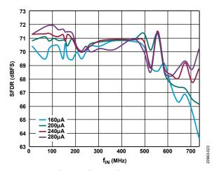
Figure 24. SFDR vs.  $f_{\rm IN}$  with Different Buffer Current Settings,  $A_{\rm IN}$  < 735 MHz
