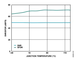
Figure 18. SNR/SFDR vs. Junction Temperature,  $f_{IN} = 611$  MHz
