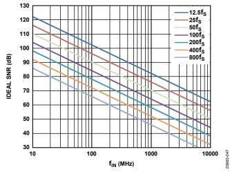
Figure 52. Ideal SNR vs. f<sub>IN</sub> over Jitter
