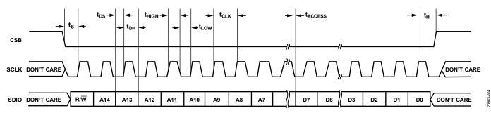
Figure 4. Serial Port Interface Timing Diagram
