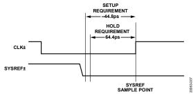
Figure 77. SYSREF $\pm$  High to Low Transition Using Rising Edge Clock Capture (Register 0x0120, Bit 4 = 1, Register 0x0120, Bit 3 = 0)
