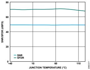
Figure 17. SNR/SFDR vs. Junction Temperature,  $f_{IN} = 155 \text{ MHz}$
