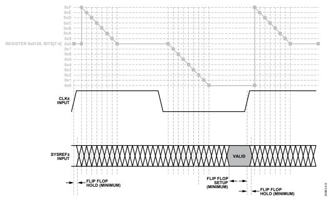
Figure 81. SYSREF $\pm$  Hold Detector
