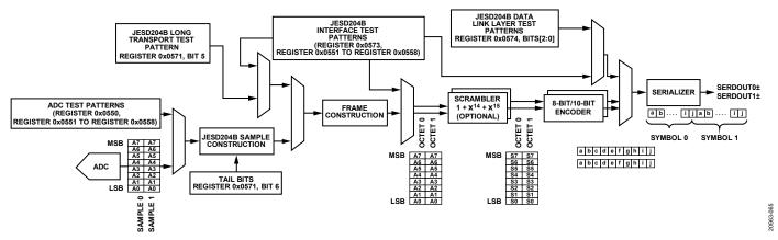
Figure 61. ADC Output Datapath with Data Framing
