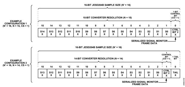
Figure 57. Signal Monitor Control Bit Locations
