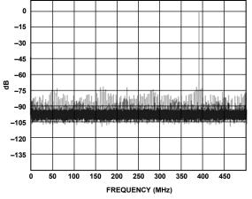
Figure 9. Single-Tone FFT with  $f_{\rm IN}$  = 611 MHz, SNRFS = 48.6 dBFS, SFDR = 71 dBFS, SINAD = 48.5 dBFS
