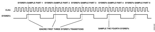
Figure 79. SYSREF± Ignore Example (SYSREF± N Shot Ignore Counter Select, Register 0x0121, Bits[3:0] = 0011)
