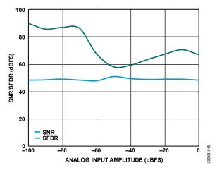
Figure 15. SNR/SFDR vs. Analog Input Amplitude,  $f_{IN} = 155 \text{ MHz}$
