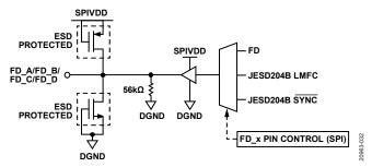
Figure 40. FD\_A, FD\_B, FD\_C, or FD\_D Outputs
