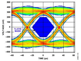
Figure 66. Digital Outputs Data Eye Diagram, External 100  $\Omega$  Terminations at 15 Gbps
