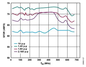
Figure 28. SFDR vs.  $f_{IN}$  with Different Analog Input Full Scales,  $A_{IN}$  < 735 MHz
