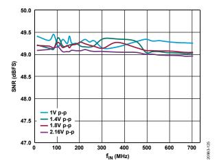
Figure 26. SNR vs.  $f_{\rm IN}$  with Different Analog Input Full Scales,  $A_{\rm IN}$  < 735 MHz
