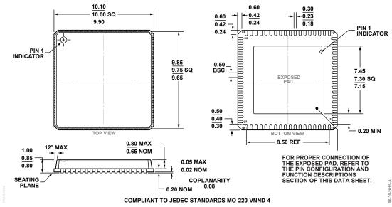
Figure 84. 72-Lead, Lead Frame Chip Scale Package [LFCSP] 10 mm × 10 mm Body and 0.85 mm Package Height (CP-72-10) Dimensions shown in millimeters
