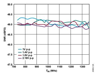
Figure 27. SNR vs.  $f_{IN}$  with Different Analog Input Full Scales,  $A_{IN} \ge 735$  MHz, Buffer Current = 320  $\mu$ A
