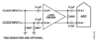
Figure 50. Differential LVDS Sample Clock
