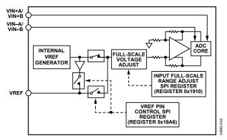
Figure 47. Internal Reference Configuration and Controls
