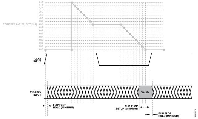
Figure 80. SYSREF± Setup Detector
