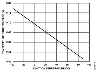
Figure 54. Temperature Diode Voltage vs. Junction Temperature
