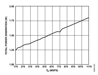
Figure 22. Total Power Dissipation vs. f<sub>s</sub>
