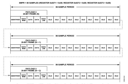
$\textit{Figure 59. SPORT over JESD204B Signal Monitor Data Example with Period Timer = 80 \, Samples}$
