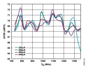
Figure 25. SFDR vs.  $f_{IN}$  with Different Buffer Current Settings,  $A_{IN} \ge 735$  MHz
