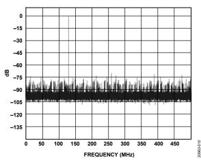
Figure 10. Single-Tone FFT with  $f_{\rm IN}$  = 871 MHz, SNRFS = 48.5 dBFS, SFDR = 70 dBFS, SINAD = 48.5 dBFS
