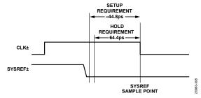
Figure 78. SYSREF $\pm$  High to Low Transition Using Falling Edge Clock Capture (Register 0x0120, Bit 4 = 1, Register 0x0120, Bit 3 = 1)
