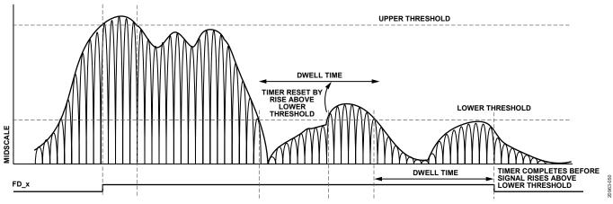
Figure 55. Threshold Settings for the FD\_x Signals
