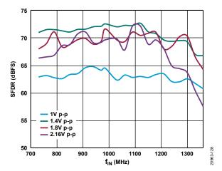
Figure 29. SFDR vs.  $f_{IN}$  with Different Analog Input Full Scales,  $A_{IN} \ge 735$  MHz, Buffer Current = 320  $\mu$ A
