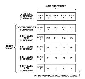
Figure 58. SPORT over JESD204B Signal Monitor Frame Data
