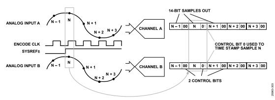
Figure 73. Timestamping, CS = 1 (Register 0x058F, Bits[7:6] = 1 Decimal), Control Bit 0 is SYSREF± (Register 0x0559, Bits[2:0] = 101)
