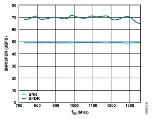
Figure 14. SNR/SFDR vs.  $f_{IN}$ ,  $A_{IN} \ge 735$  MHz, Buffer Current = 320  $\mu$ A
