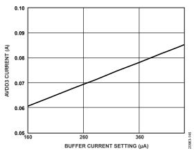
Figure 46. AVDD3 Power vs. Buffer Current Setting
