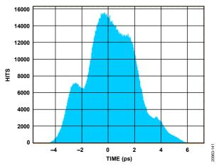
Figure 67. Digital Output TIE Jitter Histogram, External 100  $\Omega$  Terminations at 15 Gbps
