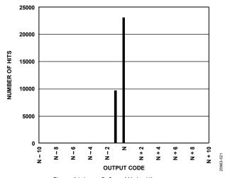
Figure 21. Input Referred Noise Histogram
