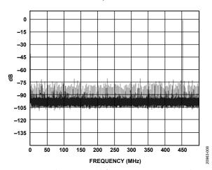
Figure 8. Single-Tone FFT with  $f_{\rm IN}$  = 451 MHz, SNRFS = 49.1 dBFS, SFDR = 71 dBFS, SINAD = 49.1 dBFS
