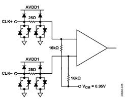
Figure 33. Clock Inputs
