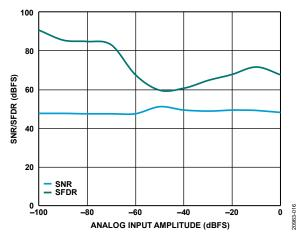
Figure 16. SNR/SFDR vs. Analog Input Amplitude,  $f_{IN} = 611$  MHz
