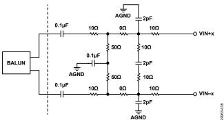
Figure 43. Differential Transformer Coupled Configuration  $A_{IN} \le 735 \text{ MHz}$
