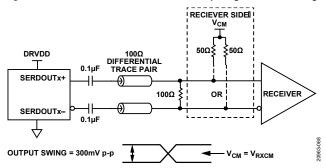
Figure 64. AC-Coupled Digital Output Termination Example (V<sub>RXCM</sub> is the Receive Side V<sub>CM</sub>)
