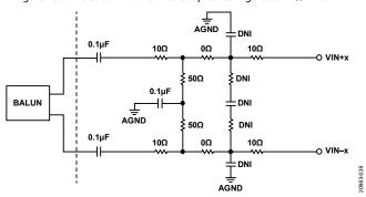
Figure 44. Differential Transformer Coupled Configuration for  $A_{IN} > 735$  MHz
