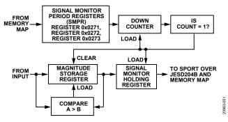
Figure 56. Signal Monitor Block
