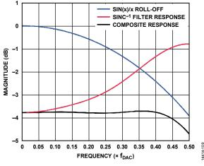
Figure 121. Responses of Sin(x)/x Roll-Off, the  $Sinc^{-1}$  Filter, and the Composite of the Two
