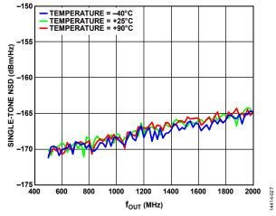
Figure 30. Single-Tone NSD Measured at 70 MHz vs. four over Temperature
