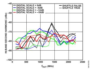
Figure 19. SFDR for In-Band Second Harmonic vs. four over Digital Scale
