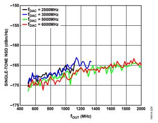
Figure 26. Single-Tone NSD Measured at 10% Offset from four vs. four over fDAC
