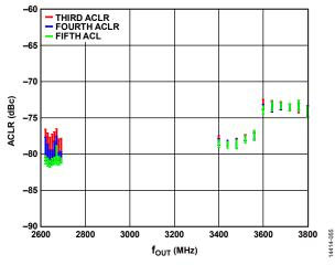
Figure 56. Single-Carrier, W-CDMA ACLR vs. four (Third ACLR, Fourth ACLR, Fifth ACLR)
