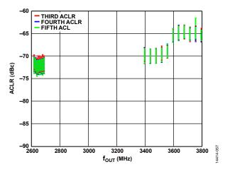
Figure 59. Four-Carrier, W-CDMA ACLR vs. fourt (Third ACLR, Fourth ACLR, Fifth ACLR)
