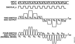
Figure 129. Two-Switch and Quad-Switch DAC Waveforms
