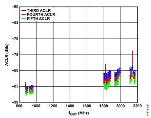
Figure 37. Single-Carrier, W-CDMA ACLR vs. four (Third ACLR, Fourth ACLR, Fifth ACLR)
