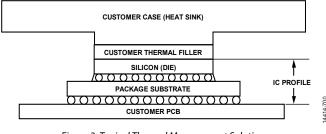
Figure 3. Typical Thermal Management Solution
