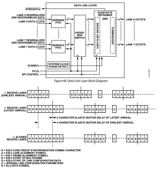
Figure 99. Lane Alignment During ILAS
