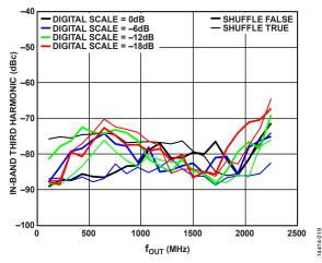
Figure 20. SFDR for In-Band Third Harmonic vs. four over Digital Scale
