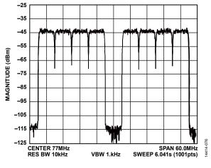
Figure 84. Gap Channel ACLR at 77 MHz
