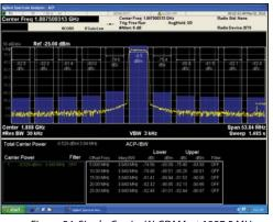
Figure 54. Single-Carrier W-CDMA at 1887.5 MHz
