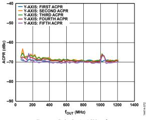
Figure 80. Eight-Carrier ACPR vs. four
