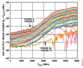
Figure 134. Performance Improvement from Tuning the Clock Input
