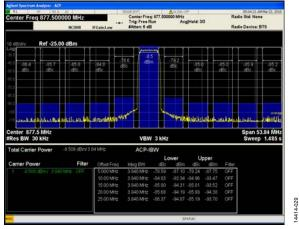
Figure 32. Single-Carrier W-CDMA at 877.5 MHz
