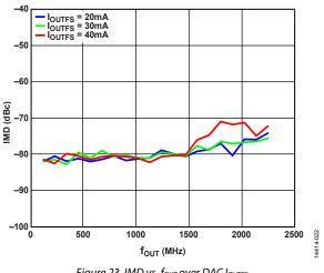
Figure 23. IMD vs. fout over DAC loutes
