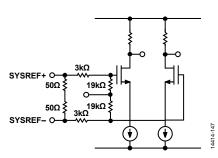
Figure 101. SYSREF± Input Circuit for the 11 mm  $\times$  11 mm 169-Ball BGA
