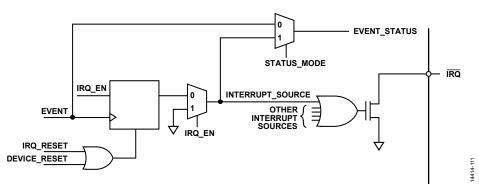
Figure 123. Simplified Schematic of IRQ Circuitry
