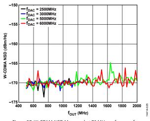
Figure 27. W-CDMA NSD Measured at 70 MHz vs. four over fDAC
