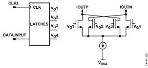
Figure 128. Quad-Switch Architecture
