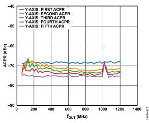
Figure 79. Four-Carrier ACPR vs. fout
