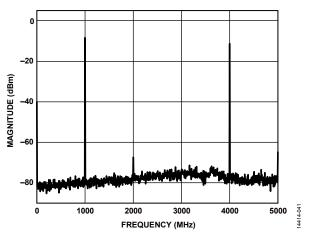
Figure 45. Single-Tone Spectrum at  $f_{OUT} = 4000 \text{ MHz}$
