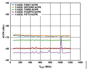
Figure 78. Single-Carrier Adjacent Channel Power Ratio (ACPR) vs.  $f_{OUT}$
