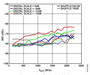
Figure 21. IMD vs. four over Digital Scale
