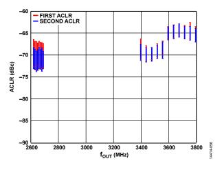
Figure 58. Four-Carrier, W-CDMA ACLR vs. four (First ACLR, Second ACLR)
