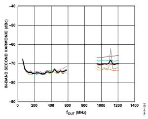
Figure 73. In-Band Second Harmonic vs. f<sub>our</sub> Performance for Four DOCSIS Carriers
