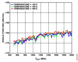
Figure 31. Single-Tone NSD Measured at 10% Offset from four vs. four over Temperature
