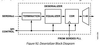
JESD204B data is input to the AD9164 via the SERDINx± 1.2 V differential input pins as per the JESD204B specification.
