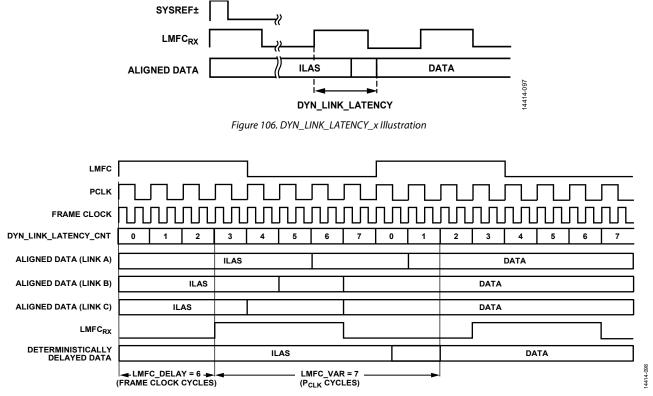
Figure 107. Multilink Synchronization Settings, Derived Method Example
