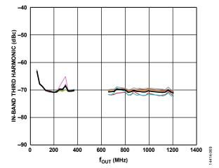
Figure 77. In-Band Third Harmonic vs. four Performance for Eight DOCSIS Carriers
