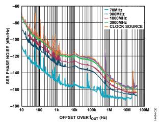
Figure 41. SSB Phase Noise vs. Offset over  $f_{OUT}$ ,  $f_{DAC} = 6000$  MSPS
