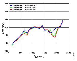
Figure 24. SFDR vs. four over Temperature
