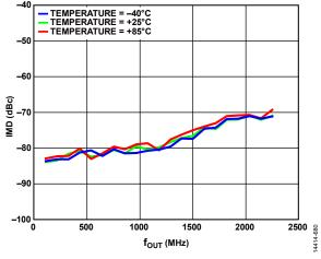
Figure 29. IMD vs. four over Temperature
