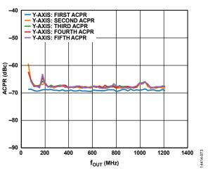
Figure 81. 16-Carrier ACPR vs. fout
