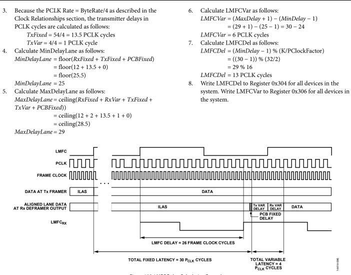
Figure 105. LMFC Delay Calculation Example
