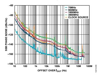
Figure 38. SSB Phase Noise vs. Offset over  $f_{OUT}$ ,  $f_{DAC}$  = 4000 MSPS (Two Different DAC Clock Sources Used for Best Composite Curve)
