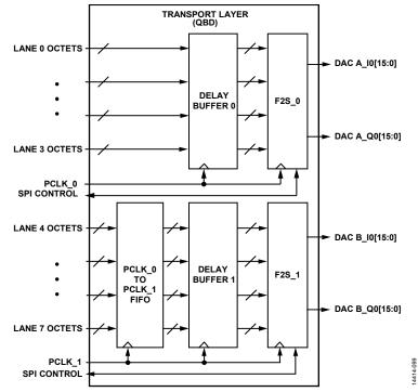
Figure 108. Transport Layer Block Diagram
