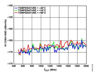
Figure 34. W-CDMA NSD Measured at 10% Offset from  $f_{OUT}$  vs.  $f_{OUT}$  over Temperature
