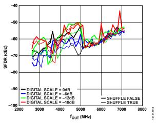
Figure 48. SFDR vs.  $f_{\text{OUT}}$  over Digital Scale
