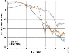
Figure 139. Measured DAC Output Response;  $f_{DAC} = 6$  GSPS
