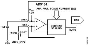
Figure 136. Voltage Reference Circuit
