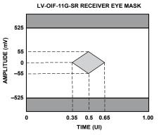
Figure 93. Receiver Eye Mask for 600 mV  $V_{\rm TT}$  Swing
