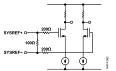
Figure 100. SYSREF $\pm$  Input Circuit for the 8 mm  $\times$  8 mm 165-Ball BGA
