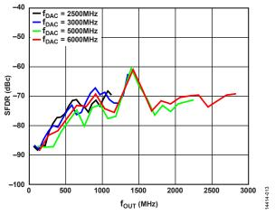
Figure 14. SFDR vs. fout over fDAC
