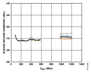
Figure 74. In-Band Second Harmonic vs. f<sub>OUT</sub> Performance for Eight DOCSIS Carriers
