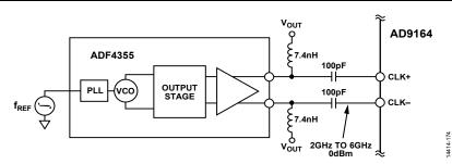
Figure 135. Possible Signal Chain for CLK± Input
