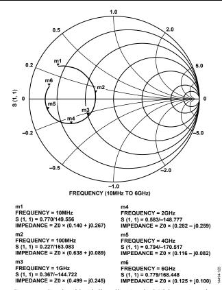
Figure 142. Simulated Smith Chart Showing the DAC Output Impedance
