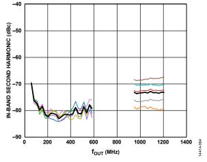
Figure 72. In-Band Second Harmonic vs.  $f_{\text{OUT}}$  Performance for One DOCSIS Carrier
