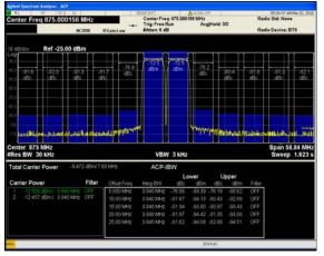
Figure 35. Two-Carrier W-CDMA at 875 MHz
