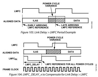
The method to select the LMFCDel (Register 0x304) and LMFCVar (Register 0x306) variables is described in the Link Delay Setup Example, with Known Delays section.
