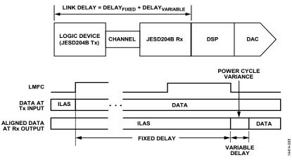
Figure 102. JESD204B Link Delay = Fixed Delay + Variable Delay
