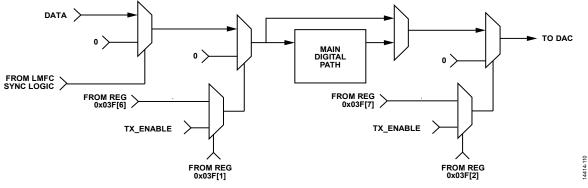
Figure 122. Downstream Protection Block Diagram
