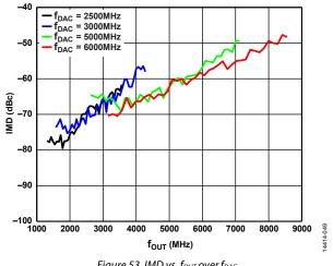
Figure 53. IMD vs. four over fDAC
