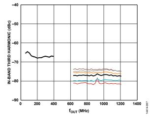
Figure 75. In-Band Third Harmonic vs. four Performance for One DOCSIS Carrier
