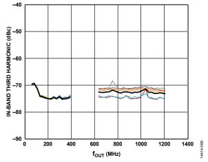
Figure 76. In-Band Third Harmonic vs. four Performance for Four DOCSIS Carriers
