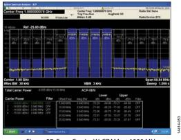
Figure 57. Four-Carrier W-CDMA at 1980 MHz
