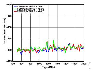
Figure 33. W-CDMA NSD Measured at 70 MHz vs.  $f_{OUT}$  over Temperature
