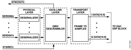
Figure 91. Functional Block Diagram of Serial Link Receiver
