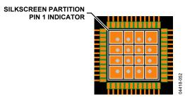
Figure 46. Typical PCB Layout
