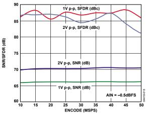
Figure 13. SNR/SFDR vs.  $f_{SAMPLE}$ ,  $f_{IN} = 10.3$  MHz,  $f_{SAMPLE} = 50$  MSPS
