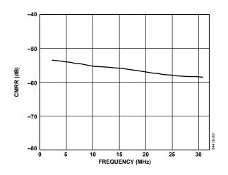
Figure 30. CMRR vs. Frequency, f<sub>SAMPLE</sub> = 65 MSPS
