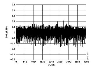
Figure 29. Typical DNL,  $f_{IN} = 2.4 \text{ MHz}$ ,  $f_{SAMPLE} = 65 \text{ MSPS}$
