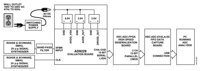
Figure 47. Evaluation Board Connections
