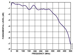
Figure 33. Full Power Bandwidth vs. Frequency,  $f_{SAMPLE} = 65 MSPS$
