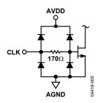
Figure 4. Equivalent Analog Input Circuit
