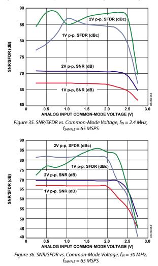
For best dynamic performance, the source impedances driving VIN+ and VIN- should be matched such that common-mode settling errors are symmetrical. These errors are reduced by the common-mode rejection of the ADC.
