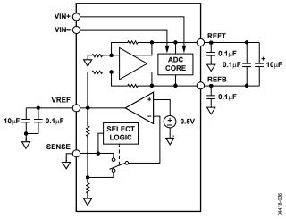
Figure 42. Internal Reference Configuration
