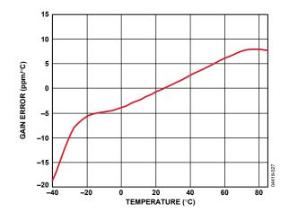
Figure 27. Gain Error vs. Temperature
