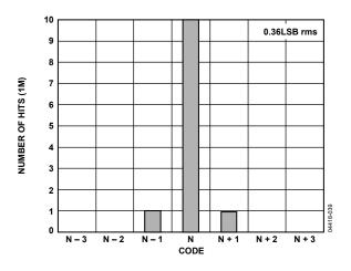
Figure 31. Input Referred Noise Histogram, f<sub>SAMPLE</sub> = 65 MSPS
