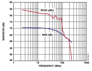
Figure 21. SNR/SFDR vs.  $f_{IN}$ ,  $f_{SAMPLE} = 65 MHz$
