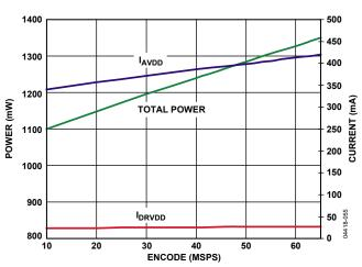
Figure 41. Supply Current vs. f<sub>SAMPLE</sub> for f<sub>IN</sub> = 10.3 MHz, f<sub>SAMPLE</sub> = 65 MSPS
