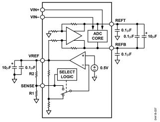
Figure 43. Programmable Reference Configuration
