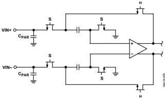
Figure 34. Switched-Capacitor SHA Input
