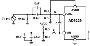
Figure 39. Single-Ended Input Configuration
