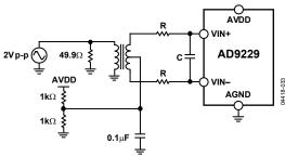
Figure 38. Differential Transformer—Coupled Configuration
