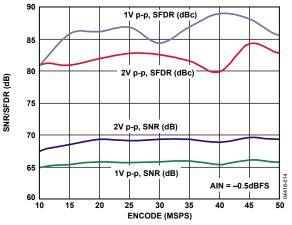
Figure 14. SNR/SFDR vs. f<sub>SAMPLE</sub>, f<sub>IN</sub> = 25 MHz, f<sub>SAMPLE</sub> = 50 MSPS
