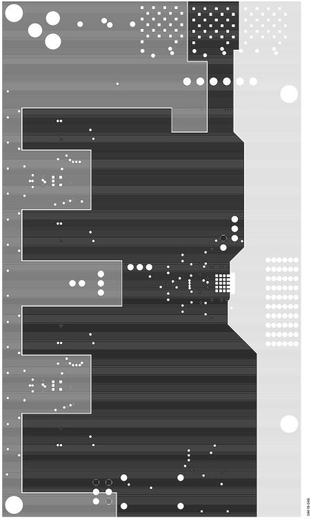
Figure 56. Evaluation Board Layout, Power Plane
