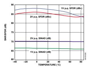
Figure 26. SINAD/SFDR vs. Temperature, f<sub>IN</sub> 10.3 MHz, f<sub>SAMPLE</sub> = 65 MSPS
