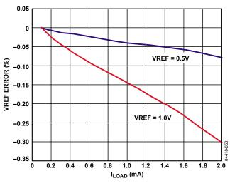
Figure 44. VREF Accuracy vs. Load
