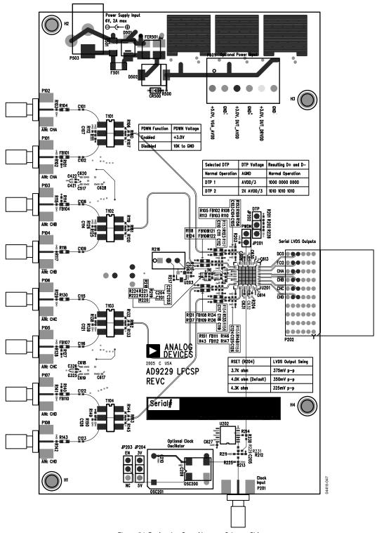
Figure 54. Evaluation Board Layout, Primary Side
