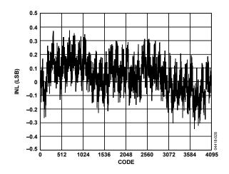
Figure 28. Typical INL,  $f_{IN} = 2.4 \text{ MHz}$ ,  $f_{SAMPLE} = 65 \text{ MSPS}$
