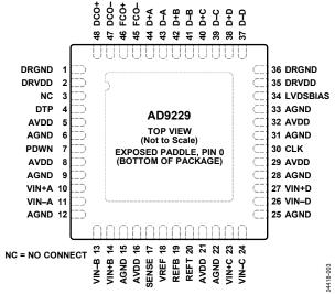
Figure 3. LFCSP Top View
