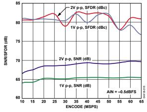
Figure 16. SNR/SFDR vs.  $f_{SAMPLE}$ ,  $f_{IN} = 30$  MHz,  $f_{SAMPLE} = 65$  MSPS
