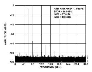
Figure 23. Two-Tone 32k FFT with  $f_{\rm IN1}$  = 69 MHz and  $f_{\rm IN2}$  = 70 MHz,  $f_{SAMPLE}$  = 65 MSPS
