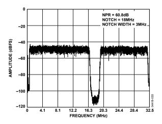
Figure 32. Noise Power Ratio (NPR),  $f_{SAMPLE} = 65 MSPS$
