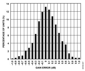
Figure 7. Gain Error Histogram, GAIN+ = 0.8 V
