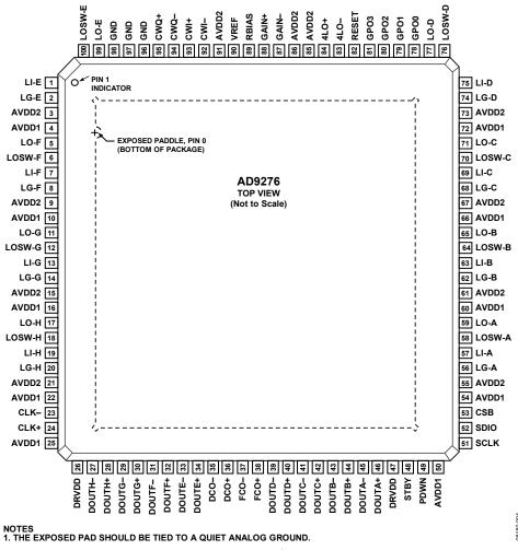
Figure 4. Pin Configuration
