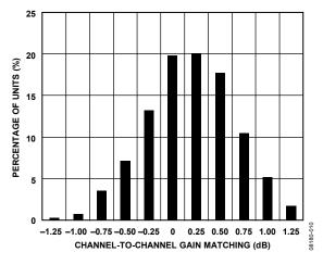
Figure 10. Gain Match Histogram, GAIN+ = 1.3 V
