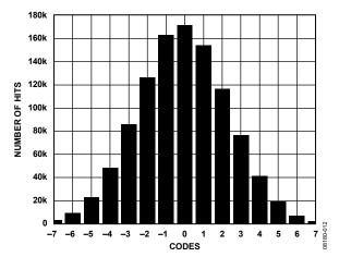
Figure 12. Output-Referred Noise Histogram, GAIN+ = 1.6 V
