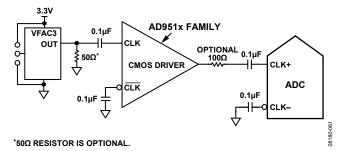
Figure 67. Single-Ended 3.3 V CMOS Sample Clock
