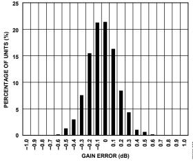
Figure 8. Gain Error Histogram, GAIN+ = 1.44 V
