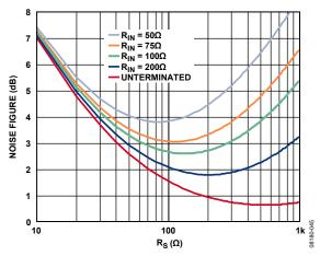
Figure 51. Noise Figure vs.  $R_S$  for Various Fixed Values of  $R_{IN}$ . Active Termination Matched Inputs,  $V_{GAIN} = 0.8 \text{ V}$
