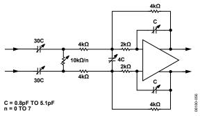
Figure 62. Simplified Antialiasing Filter Schematic
