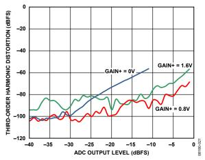
Figure 20. Third-Order Harmonic Distortion vs. ADC Output Level
