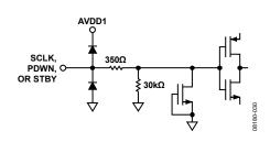
Figure 36. Equivalent SCLK, PDWN, or STBY Input Circuit
