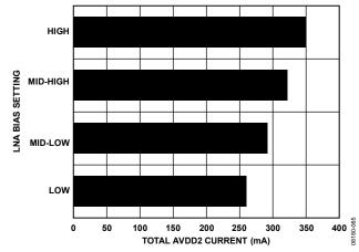
Figure 71. AVDD2 Current at Different LNA Bias Settings, f<sub>SAMPLE</sub> = 40 MSPS
