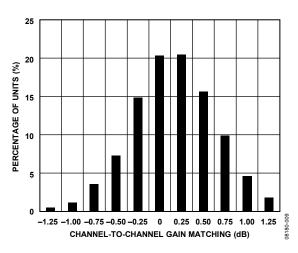
Figure 9. Gain Match Histogram, GAIN+ = 0.3 V
