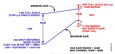
Figure 55. Gain Requirements of TGC Operation for a 12-Bit, 40 MSPS ADC
