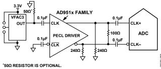
Figure 64. Differential PECL Sample Clock
