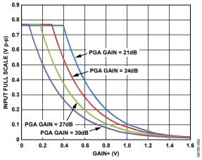
Figure 56. LNA with 15.6 dB Gain Setting/VGA Full-Scale Limitations
