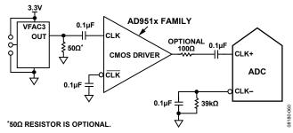
Figure 66. Single-Ended 1.8 V CMOS Sample Clock
