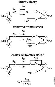
Figure 49. Input Configurations
