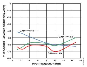
Figure 18. Third-Order Harmonic Distortion vs. Frequency, AIN = -1.0 dBFS
