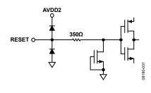
Figure 37. Equivalent RESET Input Circuit
