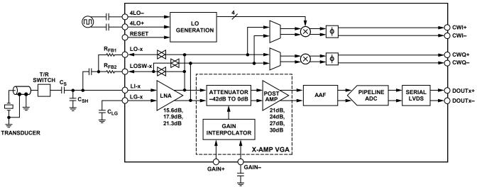
Figure 46. Simplified Block Diagram of a Single Channel
