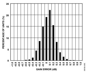
Figure 6. Gain Error Histogram, GAIN+ = 0.16 V
