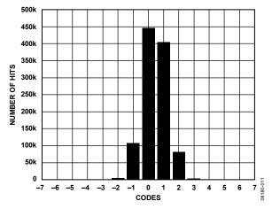
Figure 11. Output-Referred Noise Histogram, GAIN+ = 0.0 V
