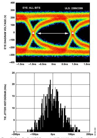
Figure 74. Data Eye for LVDS Outputs in ANSI-644 Mode with Trace Lengths of Greater Than 24 Inches on Standard FR-4
