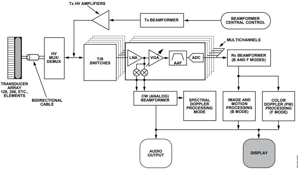
Figure 45. Simplified Ultrasound System Block Diagram
