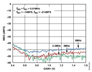
Figure 21. IMD3 vs. GAIN+
