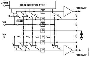
Figure 59. Simplified VGA Schematic
