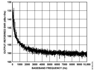
Figure 28. Output-Referred SNR vs. Baseband Frequency
