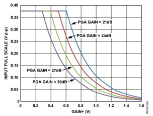
Figure 58. LNA with 21.3 dB Gain Setting/VGA Full-Scale Limitations
