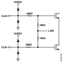
Figure 32. Equivalent Clock Input Circuit
