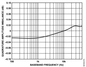
Figure 24. Quadrature Amplitude Imbalance vs. Baseband Frequency
