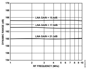
Figure 29. Small-Signal Dynamic Range vs. RF Frequency
