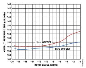
Figure 25. Output-Referred SNR vs. Input Level
