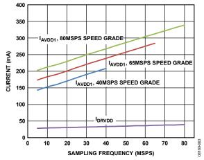
Figure 69. Supply Current vs.  $f_{SAMPLE}$  for  $f_{IN} = 5$  MHz
