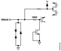
Figure 40. Equivalent RBIAS Circuit
