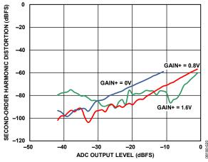
Figure 19. Second-Order Harmonic Distortion vs. ADC Output Level
