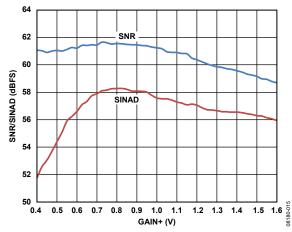
Figure 15. SNR/SINAD vs. GAIN+, AIN = -1.0 dBFS
