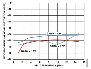
Figure 17. Second-Order Harmonic Distortion vs. Frequency, AIN = -1.0 dBFS
