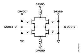
Figure 35. Equivalent Digital Output Circuit
