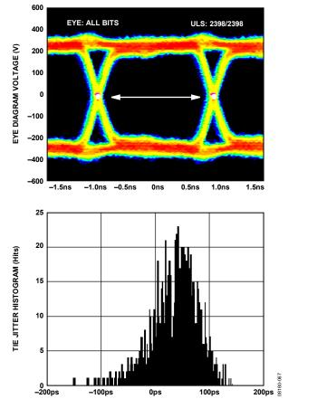
Figure 73. Data Eye for LVDS Outputs in ANSI-644 Mode with Trace Lengths of Less Than 24 Inches on Standard FR-4
