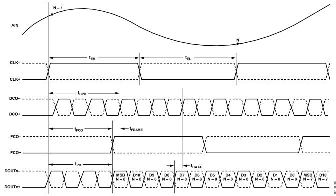
Figure 2. 12-Bit Data Serial Stream (Default)
