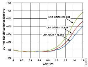
Figure 14. Short-Circuit, Output-Referred Noise vs. GAIN+
