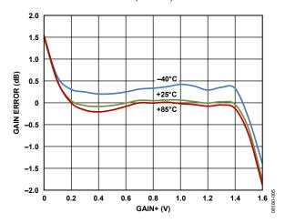
Figure 5. Gain Error vs. GAIN+ at Three Temperatures
