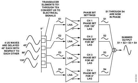
Figure 54. Simplified Example of the AD9276 Phase Shifter
