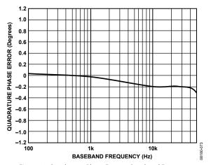
Figure 23. Quadrature Phase Error vs. Baseband Frequency
