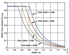
Figure 57. LNA with 17.9 dB Gain Setting/VGA Full-Scale Limitations
