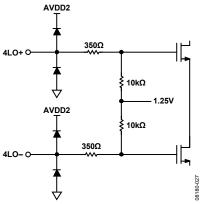
Figure 33. Equivalent 4LO Input Circuit
