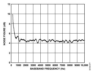
Figure 27. Noise Figure vs. Baseband Frequency
