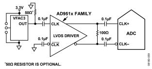
Figure 65. Differential LVDS Sample Clock
