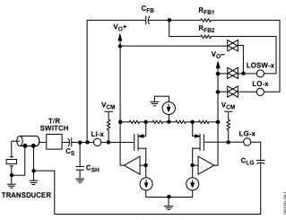
Figure 47. Simplified LNA Schematic
