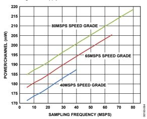
Figure 70. Power per Channel vs.  $f_{SAMPLE}$  for  $f_{IN} = 5$  MHz
