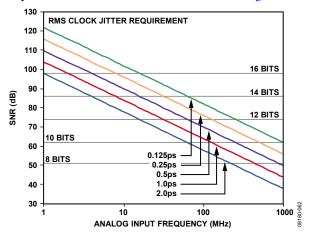
Figure 68. Ideal SNR vs. Input Frequency and Jitter
