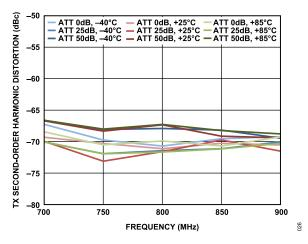
Figure 26. TX Second-Order Harmonic Distortion vs. Frequency
