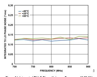
Figure 24. Integrated TX LO Phase Noise vs. Frequency, 30.72 MHz Reference Clock (Doubled Internally for RF Synthesizer)
