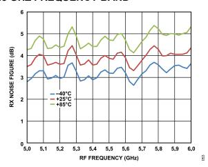
Figure 53. RX Noise Figure vs. RF Frequency
