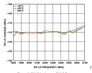
Figure 40. RX LO Leakage vs. RX LO Frequency
