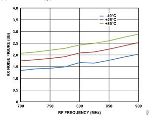
Figure 3. RX Noise Figure vs. RF Frequency
