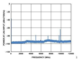
Figure 41. Power at LNA Input vs. Frequency, DC to 12 GHz,  $f_{LO\_RX}$  = 2.4 GHz, LTE 20 MHz,  $f_{LO\_TX}$  = 2.46 GHz
