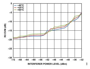
Figure 8. RX EVM vs. Interferer Power Level, LTE 10 MHz Signal of Interest withInput Power (P<sub>IN</sub>) = −82 dBm, 5 MHz Orthogonal Frequency Division Multiplexing (OFDM) Blocker at 7.5 MHz Offset
