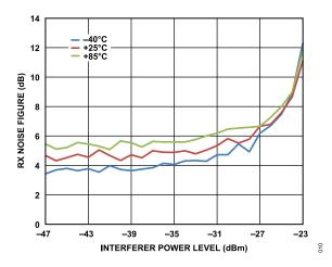
Figure 10. RX Noise Figure vs. Interferer Power Level, Edge Signal of Interest with  $P_{\rm IN}$  = -90 dBm, Continuous Wave Blocker at 3 MHz Offset, Gain Index = 64
