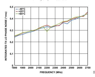
Figure 46. Integrated TX LO Phase Noise vs. Frequency, 40 MHz Reference Clock
