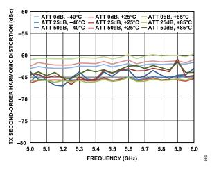
Figure 63. TX Second-Order Harmonic Distortion vs. Frequency
