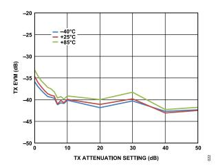
Figure 22. TX EVM vs. TX Attenuation Setting,  $f_{\rm LO\_TX}$  = 800 MHz, GSM Modulation, 30.72 MHz Reference Clock (Doubled Internally for RF Synthesizer)
