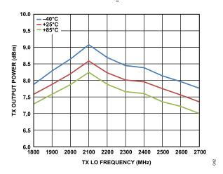
Figure 42. TX Output Power vs. TX LO Frequency, Attenuation Setting = 0 dB, Single-Tone Output
