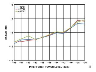
Figure 9. RX EVM vs. Interferer Power Level, LTE 10 MHz Signal of Interest with  $P_{\rm IN}$  = -90 dBm, 5 MHz OFDM Blocker at 17.5 MHz Offset
