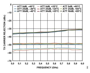
Figure 62. TX Carrier Rejection vs. Frequency
