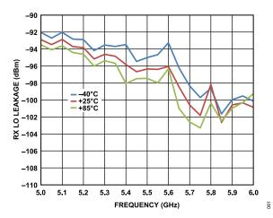
Figure 58. RX LO Leakage vs. Frequency
