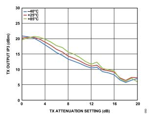
Figure 50. TX OIP3 vs. TX Attenuation Setting
