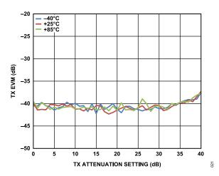
Figure 21. TX EVM vs. TX Attenuation Setting,  $f_{\rm LO\_TX}$  = 800 MHz, LTE 10 MHz, 64 QAM Modulation, 19.2 MHz Reference Clock
