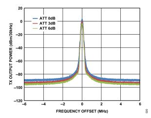
Figure 20. TX Output Power vs. Frequency Offset from Carrier Frequency,  $f_{\text{LO\_TX}}$  = 800 MHz, GSM Downlink (Digital Attenuation Variations Shown), 12 MHz Range
