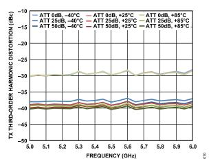
Figure 64. TX Third-Order Harmonic Distortion vs. Frequency
