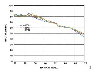
Figure 13. IIP2 vs. RX Gain Index, f1 = 2.00 MHz, f2 = 2.01 MHz, GSM Mode
