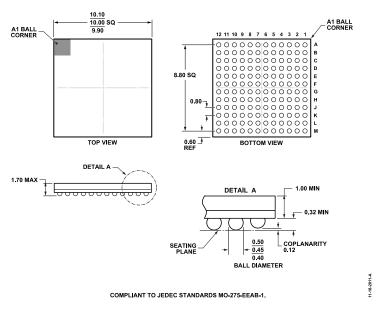
Figure 67. 144-Ball Chip Scale Package Ball Grid Array [CSP\_BGA]
