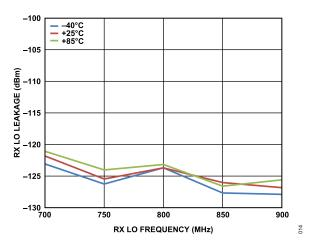
Figure 14. RX LO Leakage vs. RX LO Frequency
