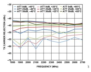
Figure 47. TX Carrier Rejection vs. Frequency
