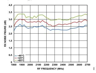
Figure 32. RX Noise Figure vs. RF Frequency
