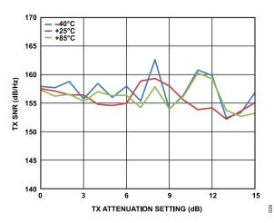
Figure 29. TX SNR vs. TX Attenuation Setting, LTE 10 MHz Signal of Interest with Noise Measured at 90 MHz Offset
