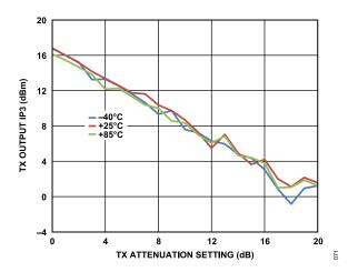
Figure 65. TX OIP3 vs. TX Attenuation Setting,  $f_{\text{LO\_TX}} = 5.8 \text{ GHz}$
