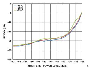
Figure 35. RX EVM vs. Interferer Power Level, LTE 20 MHz Signal of Interest with  $P_{\rm IN}$  = -75 dBm, LTE 20 MHz Blocker at 20 MHz Offset
