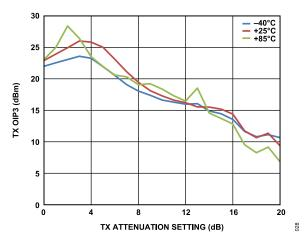
Figure 28. TX OIP3 vs. TX Attenuation Setting
