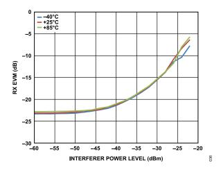
Figure 36. RX EVM vs. Interferer Power Level, LTE 20 MHz Signal of Interest with  $P_{\rm IN}$  = -75 dBm, LTE 20 MHz Blocker at 40 MHz Offset
