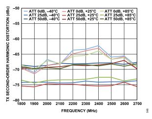
Figure 48. TX Second-Order Harmonic Distortion vs. Frequency
