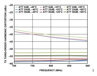
Figure 27. TX Third-Order Harmonic Distortion vs. Frequency
