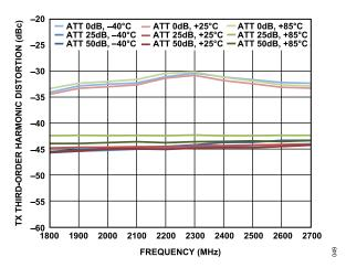
Figure 49. TX Third-Order Harmonic Distortion vs. Frequency
