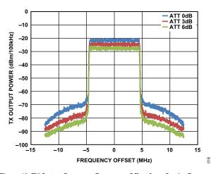
Figure 18. TX Output Power vs. Frequency Offset from Carrier Frequency,  $f_{\text{LO\_TX}}$  = 800 MHz, LTE 10 MHz Downlink (Digital Attenuation Variations Shown)
