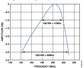
Figure 7. Antialiasing Filter Response,  $f_C = 203$  MHz, 1 dB and 3 dB Bandwidth
