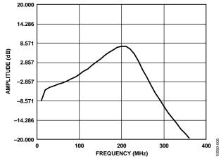
Figure 6. Antialiasing Filter Response,  $f_c = 203 \text{ MHz}$
