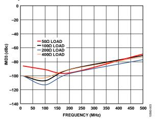
Figure 3. ADL5565 IMD3 vs. Frequency for 50  $\Omega$ , 100  $\Omega$ , 200  $\Omega$ , and 400  $\Omega$ Output Loads, 3.3 V Supply, Gain = 6 dB
