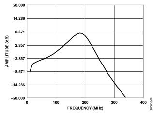
Figure 9. Antialiasing Filter Response,  $f_C = 183 \text{ MHz}$
