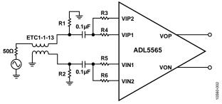
Figure 2. ADL5565 Input Impedance Match
