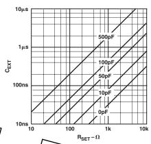
Figure 4. RC Values vs. Full-Scale Delay Range ( $t_{DFS}$ )
