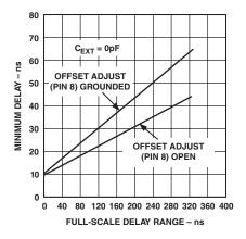
Figure 3. Minimum Delay (t<sub>PD</sub>) vs. Full-Scale Delay Range (t<sub>DFS</sub>)
