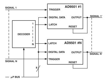
Figure 7. Multiple Signal Path Deskewing
