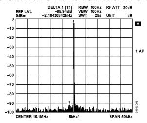
Figure 4. DAC Performance: 400 MSPS Clock, 10 MHz F<sub>ΟυΤ</sub>, 50 kHz Span
