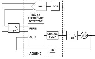
Figure 35. Direct Upconversion of DDS Output Spectrum
