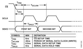
Figure 43. Timing Diagram for Data Write to AD9540
