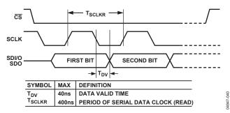
Figure 44. Timing Diagram for Data Read from AD9540
