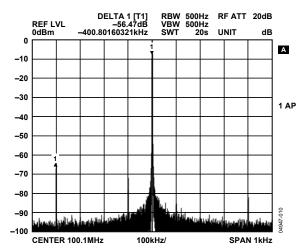
Figure 11. DAC Performance: 400 MSPS Clock, 100 MHz F<sub>OUT</sub>, 1 MHz Span
