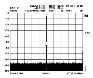
Figure 12. DAC Performance: 400 MSPS Clock, 100 MHz F<sub>ОИТ</sub>, 200 MHz Span
