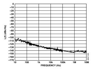
Figure 18. DDS/DAC Residual Phase Noise 400 MHz Clock, 105.3 MHz Output
