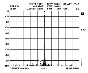
Figure 13. DAC Performance: 400 MSPS Clock, 160 MHz F<sub>ΟUT</sub>, 50 kHz Span
