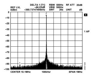
Figure 5. DAC Performance: 400 MSPS Clock, 10 MHz F<sub>OUT</sub>, 1 MHz Span
