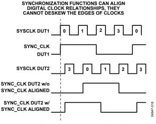
Figure 38. Synchronization Functions: Capabilities and Limitations
