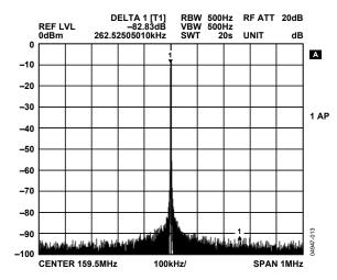
Figure 14. DAC Performance: 400 MSPS Clock, 160 MHz F<sub>OUT</sub>, 1 MHz Span
