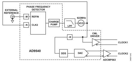
Figure 33. Optical Networking Clock
