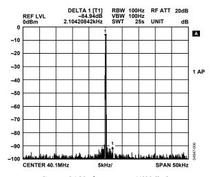
Figure 7. DAC Performance: 400 MSPS Clock, 40 MHz F<sub>OUT</sub>, 50 kHz Span
