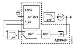
Figure 34. Fractional-Divider Loop
