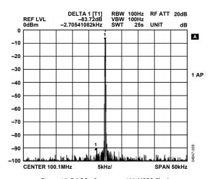
Figure 10. DAC Performance: 400 MSPS Clock, 100 MHz  $F_{\text{OUT}}$ , 50 kHz Span
