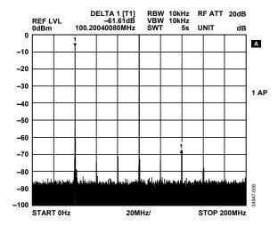
Figure 9. DAC Performance: 400 MSPS Clock, 40 MHz F<sub>OUT</sub>, 200 MHz Span (Nyquist)
