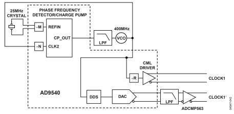
Figure 32. Dual Clock Configuration
