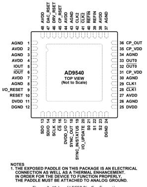
Figure 3. 48-Lead LFCSP Pin Configuration
