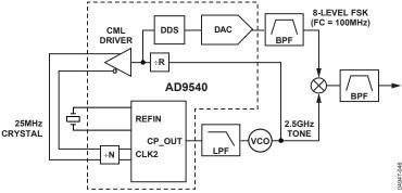
Figure 36. ISM Band Modulator (LO & Baseband Generation)
