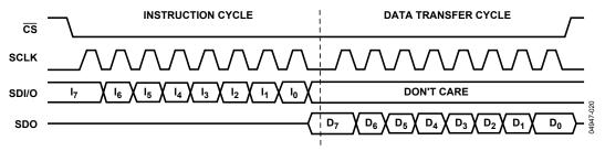
Figure 40. 3-Wire Serial Port Read Timing—Clock Stall Low
