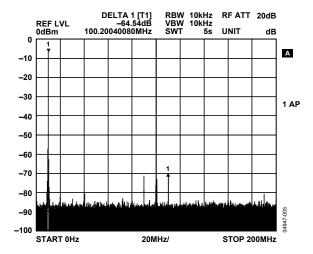
Figure 6. DAC Performance: 400 MSPS Clock, 10 MHz F<sub>OUT</sub>, 200 MHz Span
