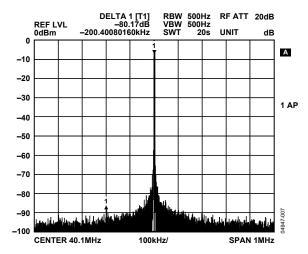
Figure 8. DAC Performance: 400 MSPS Clock, 40 MHz F<sub>OUT</sub>, 1 MHz Span
