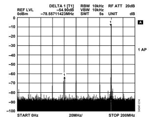
Figure 15. DAC Performance: 400 MSPS Clock, 160 MHz F<sub>OUT</sub>, 200 MHz Span
