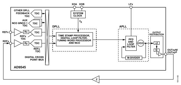
Figure 71. External Zero Delay PLL Configuration
