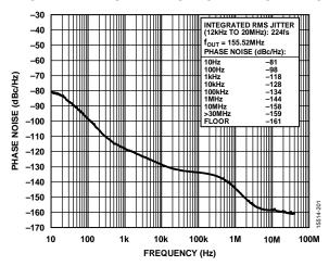
Figure 3. Absolute Phase Noise (PLL0, Configuration 1, HCSL Mode,  $f_{REF} = 38.88$  MHz,  $f_{OUT} = 155.52$  MHz,  $f_{OSC} = 52$  MHz Crystal, 50 Hz DPLL BW
