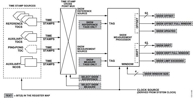
Figure 95. Skew Measurement Block Diagram
