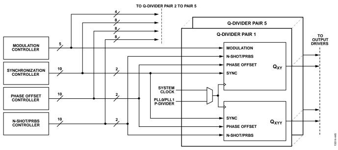
Figure 53. Functional Block Diagram of Q-Dividers and Controllers
