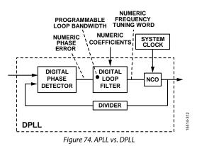
The DPLLs in the AD9545 have a digital TDC-based phase detector and a digital loop filter with programmable bandwidth. The digital loop filter output yields a digital FTW (instead of a dc voltage, as in the case of an analog PLL) that produces a corresponding NCO output frequency.
