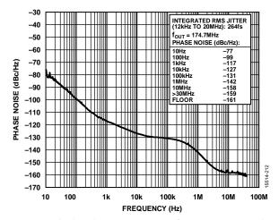
Figure 14. Absolute Phase Noise (PLL1, Configuration 6, HCSL Mode, f<sub>REF</sub> = 155.52 MHz, f<sub>OUT</sub> = 174.7 MHz, f<sub>OSC</sub> = 52 MHz Crystal, 50 Hz DPLL BW, Phase Buildout Mode)
