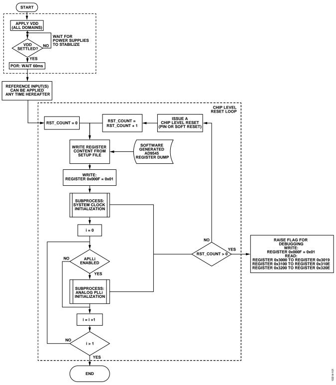
Figure 119. Programming Sequence Loop
