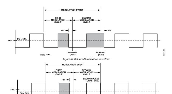
Figure 63. Unbalanced Modulation Waveform
