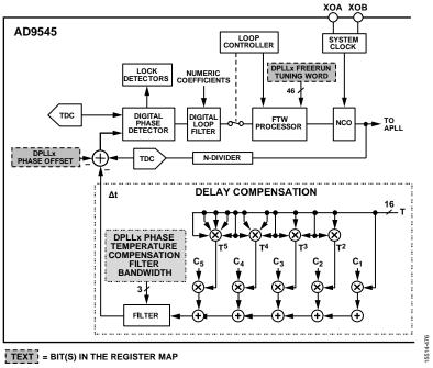
Figure 83. Delay Compensation
