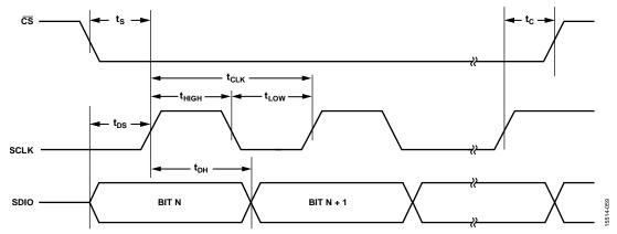
Figure 127. Serial Control Port Timing—Write
