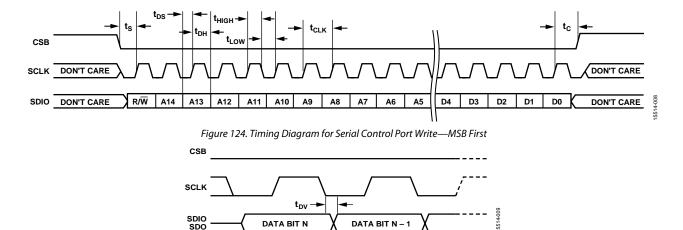
Figure 125. Timing Diagram for Serial Control Port Register Read—MSB First
