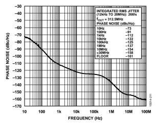
Figure 13. Absolute Phase Noise (PLL1, Configuration 5, HCSL Mode,  $f_{REF} = 25$  MHz,  $f_{OUT} = 312.5$  MHz,  $f_{OSC} = 52$  MHz Crystal, 50 Hz DPLL BW, Phase Buildout Mode)
