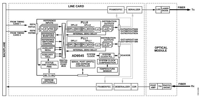
Figure 115. Optical Line Card Direct Timing Example
