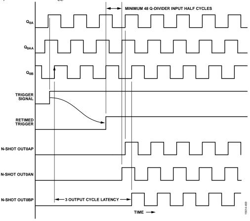
Figure 67. Trigger Retiming (with  $Q_{\text{OAA}}$  as the Retiming Q-Divider)
