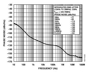
Figure 4. Absolute Phase Noise (PLL0, Configuration 2, HCSL Mode,  $f_{REF} = 30.72$  MHz,  $f_{OUT} = 245.76$  MHz,  $f_{OSC} = 52$  MHz Crystal, 50 Hz DPLL BW)
