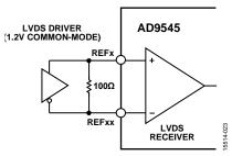
Figure 34. Differential LVDS Input Mode
