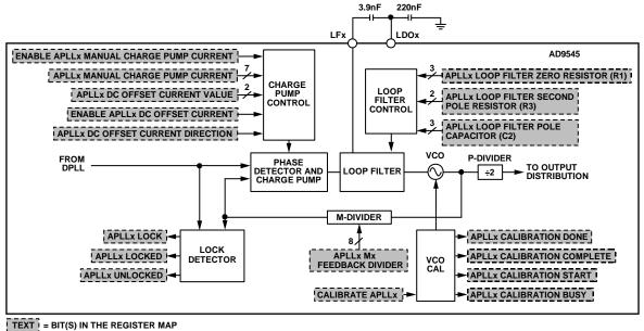
Figure 86. APLL Block Diagram
