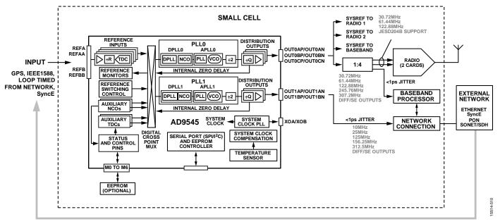
Figure 117. AD9545 Small Cell Application
