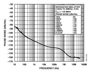
Figure 6. Absolute Phase Noise (PLL0, Configuration 4, HCSL Mode,  $f_{REF} = 125$  MHz,  $f_{OUT} = 125.0$  MHz,  $f_{COMP} = 19.2$  MHz TCXO,  $f_{OSC} = 52$  MHz Crystal, 0.1 Hz DPLL BW, Phase Buildout Mode)
