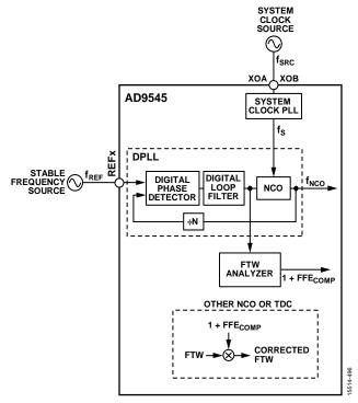
Figure 103. Closed-Loop Method
