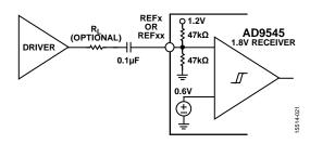
Figure 32. Single-Ended AC-Coupled Interface Mode
