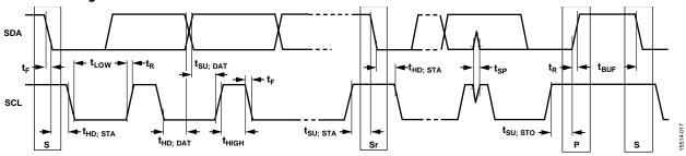
Figure 133. I<sup>2</sup>C Serial Port Timing
