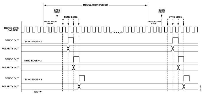
Figure 52. Demodulation Synchronization
