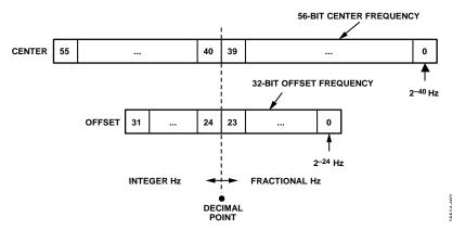
Figure 99. Auxiliary NCO Frequency Tuning
