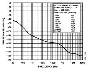
Figure 7. Absolute Phase Noise (PLL0, Configuration 5, HCSL Mode,  $f_{REF} = 25$  MHz,  $f_{OUT} = 312.5$  MHz,  $f_{OSC} = 52$  MHz Crystal, 50 Hz DPLL BW, Phase Buildout Mode)
