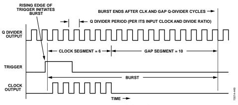
Figure 57. Burst Clock Signal
