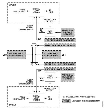
Figure 76. Digital Loop Filter Block Diagram
