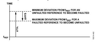
Figure 50. Reference Monitor Fault and Unfault Parameters
