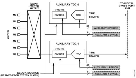
Figure 96. Auxiliary TDC Block Diagram
