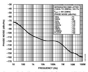
Figure 11. Absolute Phase Noise (PLL1, Configuration 3, HCSL Mode,  $f_{REF} = 1$  Hz,  $f_{OUT} = 491.52$  MHz,  $f_{COMP} = 19.2$  MHz TCXO,  $f_{OSC} = 52$  MHz Crystal, 0.05 Hz DPLL BW)
