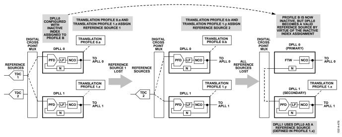
Figure 85. Cascaded DPLL Configuration
