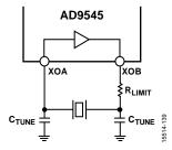
Figure 48. Power Limiting Resistor Connection
