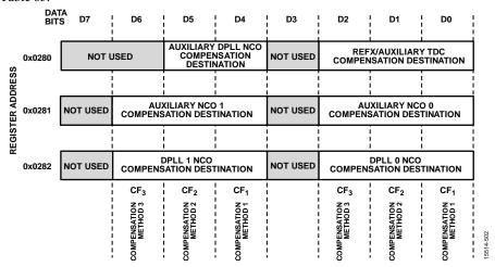
Figure 109. System Clock Compensation Registers
