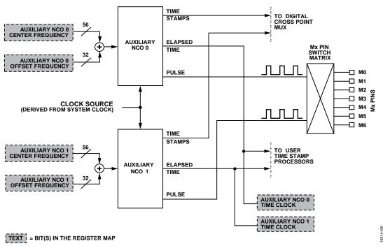
Figure 98. Auxiliary NCO Block Diagram
