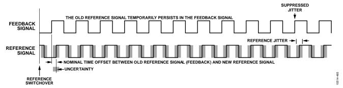
Figure 73. DPLL Reference and Feedback Signals
