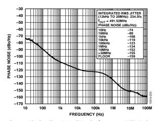
Figure 5. Absolute Phase Noise (PLL0, Configuration 3, HCSL Mode,  $f_{REF} = 1$  Hz,  $f_{OUT} = 491.52$  MHz,  $f_{COMP} = 19.2$  MHz TCXO,  $f_{OSC} = 52$  MHz Crystal, 0.05 Hz DPLL BW)
