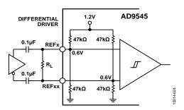
Figure 35. Differential AC-Coupled Mode ( $R_L = 100 \Omega$  Is Recommended, Except For HCSL)
