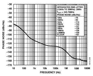
Figure 10. Absolute Phase Noise (PLL1, Configuration 2, HCSL Mode,  $f_{REF} = 30.72$  MHz,  $f_{OUT} = 245.76$  MHz,  $f_{OSC} = 52$  MHz Crystal, 50 Hz DPLL BW)
