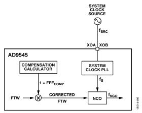
Figure 102. Open-Loop Method
