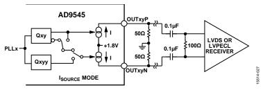
Figure 37. LVDS-Compatible Output Swing, AC-Coupled (375 mV (Differential) Across 100  $\Omega$  Termination Resistor for I = 15 mA)
