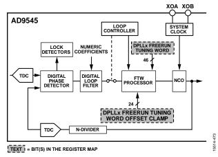
Figure 81. Tuning Word Offset Clamp Feature
