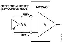
Figure 36. Differential DC-Coupled Mode
