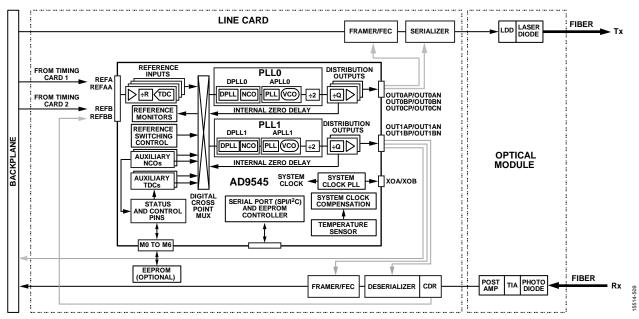
Figure 116. Optical Line Card Loop Timing Example
