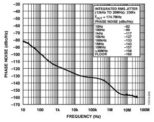
Figure 8. Absolute Phase Noise (PLL0, Configuration 6, HCSL Mode,  $f_{REF} = 155.52$  MHz,  $f_{OUT} = 174.7$  MHz,  $f_{OSC} = 52$  MHz Crystal, 50 Hz DPLL BW, Phase Buildout Mode)
