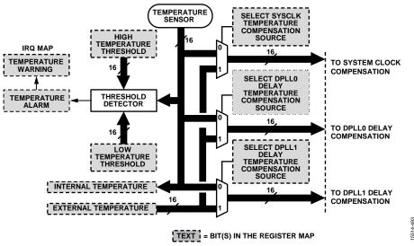
Figure 100. Temperature Sensor Block Diagram
