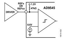
Figure 33. Single-Ended Internal Pull-Up Resistor Mode
