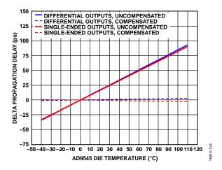
Figure 24. DPLL Delay Compensation vs. Temperature; Differential AC-Coupled Input Reference Mode (HSTL Levels); f<sub>SYS</sub> = 2392 MHz; Internal Zero Delay (Hitless) Mode
