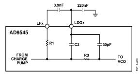
Figure 87. APLL Loop Filter
