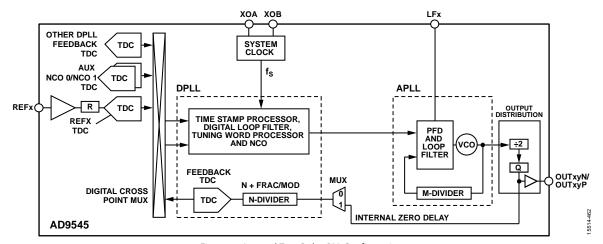
Figure 70. Internal Zero Delay PLL Configuration
