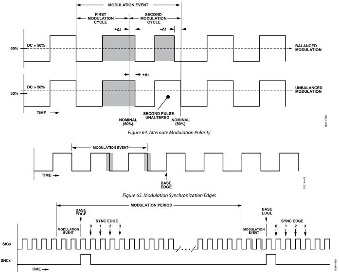
Figure 66. Modulation Synchronization
