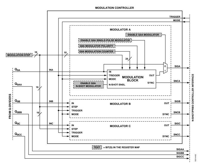
Figure 60. Block Diagram of Embedded Clock Modulation Controller
