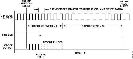
Figure 59. Stalling a Periodic Gapped Clock Signal
