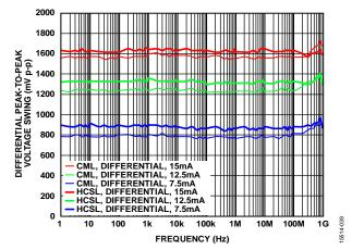
Figure 20. Differential Peak-to-Peak Voltage Swing vs. Frequency; HCSL Drivers Terminated 50  $\Omega$  to GND per Figure 38; CML Drivers Terminated 50  $\Omega$  to 1.8 V per Figure 39
