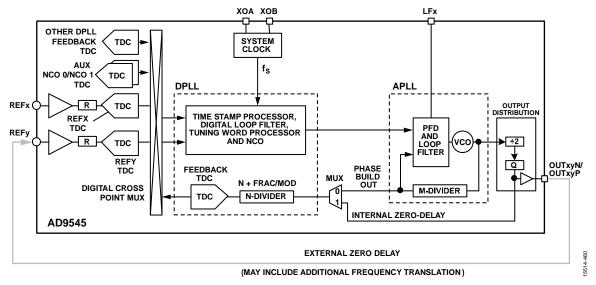
Figure 68. Frequency Translation Loop Block Diagram
