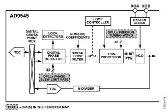
Figure 82. Phase Slew Limit Feature
