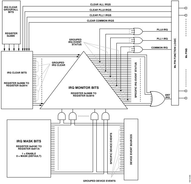
Figure 111. IRQ System Diagram
