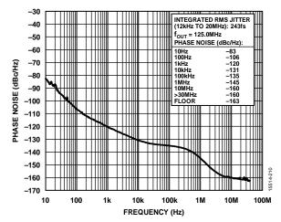
Figure 12. Absolute Phase Noise (PLL1, Configuration 4, HCSL Mode,  $f_{REF} = 125$  MHz,  $f_{OUT} = 125$  MHz,  $f_{COMP} = 19.2$  MHz TCXO,  $f_{OSC} = 52$  MHz Crystal, 0.1 Hz DPLL BW, Phase Buildout Mode)
