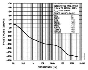
Figure 9. Absolute Phase Noise (PLL1, Configuration 1, HCSL Mode,  $f_{REF} = 38.88$  MHz,  $f_{OUT} = 155.52$  MHz,  $f_{OSC} = 52$  MHz Crystal, 50 Hz DPLL BW)
