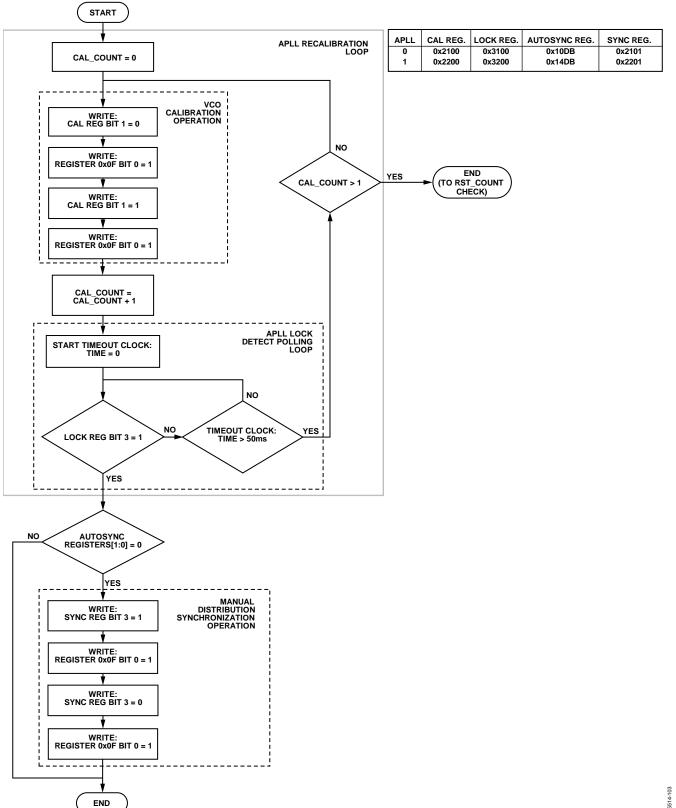
Figure 121. AD9545 Analog PLL Initialization Subprocess
