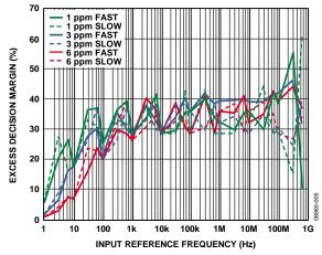
Figure 5. Excess Decision Margin for Tolerance = 1 ppm, 3 ppm, and 6 ppm
