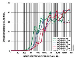
Figure 8. Excess Decision Margin for Tolerance = 1000 ppm, 3000 ppm, and 6000 ppm
