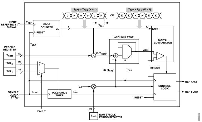
Figure 2. Reference Monitor Detailed Block Diagram
