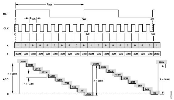
Figure 3. Accumulator Output Waveform for  $T_{REF} > T_{CLK}$
