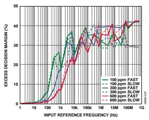
Figure 7. Excess Decision Margin for Tolerance = 100 ppm, 300 ppm, and 600 ppm
