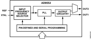
Figure 1. Simplified Block Diagram of AD9552 Oscillator Frequency Upconverter
