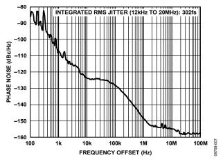
Figure 7. Absolute Phase Noise (Output Driver = 3.3.V CMOS),  $f_R = 19.44$  MHz,  $f_{OUT} = 161.1328125$  MHz, DPLL Loop BW = 100 Hz,  $f_{SYS} = 49.152$  MHz Crystal
