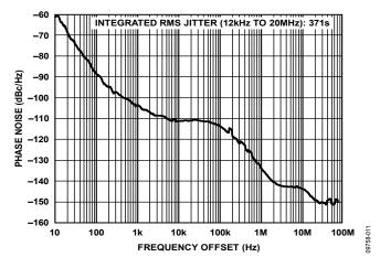
Figure 11. Absolute Phase Noise (Output Driver = HSTL),  $f_R = 19.44$  MHz,  $f_{OUT} = 693.482991$  MHz, DPLL Loop BW = 0.1 Hz,  $f_{SYS} = 19.2$  MHz TCXO
