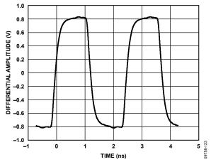
Figure 23. Output Waveform, HSTL (400 MHz)
