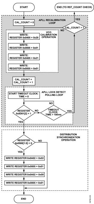
Figure 37. AD9558 APLL Initialization Subprocess Flowchart
