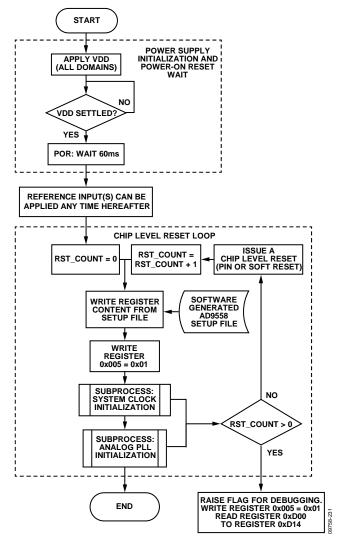
Figure 35. AD9558 Initialization Flowchart
