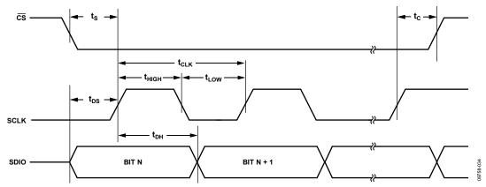
Figure 54. Serial Control Port Timing—Write
