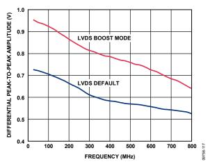
Figure 17. Amplitude vs. Toggle Rate, LVDS
