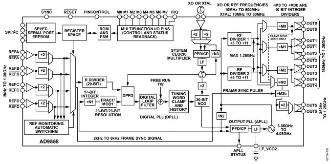
Figure 38. Detailed Block Diagram
