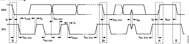
Figure 60. I<sup>2</sup>C Serial Port Timing
