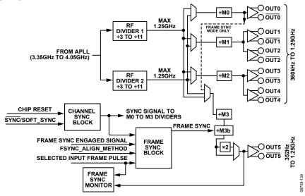
Figure 43. Clock Distribution Block Diagram
