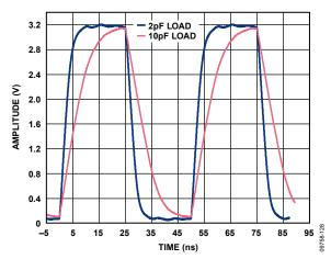
Figure 27. Output Waveform, 3.3 V CMOS (20 MHz, Weak Mode)
