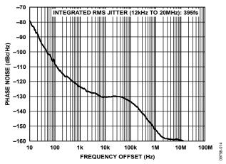
Figure 14. Absolute Phase Noise (Output Driver = 1.8 V CMOS),  $f_R = 2 \text{ kHz}, f_{\text{OUT}} = 70.656 \text{ MHz}, \\ DPLL Loop BW = 0.1 \text{ Hz}, f_{\text{SYS}} = 19.2 \text{ MHz TCXO}$
