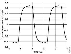
Figure 24. Output Waveform, LVDS (400 MHz)
