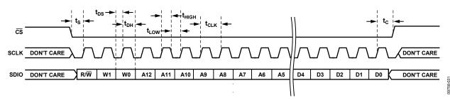
Figure 51. Serial Control Port Write—MSB First, 16-Bit Instruction, Timing Measurements
