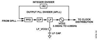
Figure 42. Output PLL Block Diagram
