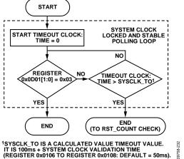
Figure 36. AD9558 System Clock Initialization Subprocess Flowchart
