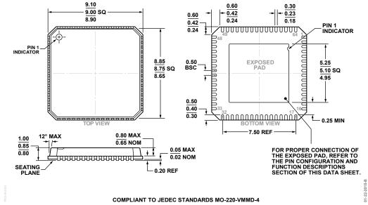
Figure 61. 64-Lead Lead Frame Chip Scale Package [LFCSP\_VQ] 9 mm × 9 mm Body, Very Thin Quad (CP-64-5) Dimensions shown in millimeters
