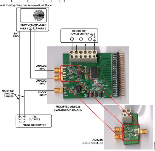
Figure 7. Converter Input Impedance Measurement Setup
