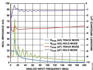
Figure 10. Differential Input Impedance vs. Analog Input Frequency (Expanded)
