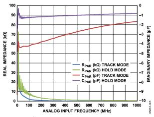
Figure 9. Differential Input Impedance vs. Analog Input Frequency
