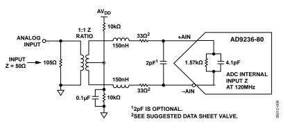
Figure 11. Impedance Matching Example
