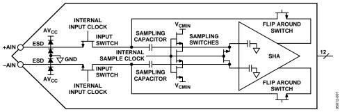
Figure 1. Unbuffered Converter Input Front-End Model
