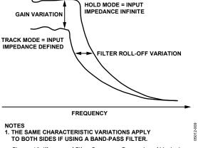
Figure 12. Illustrated Filter Response Due to Load Variation
