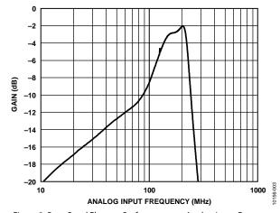
Figure 3. Pass-Band Flatness Performance vs. Analog Input Frequency
