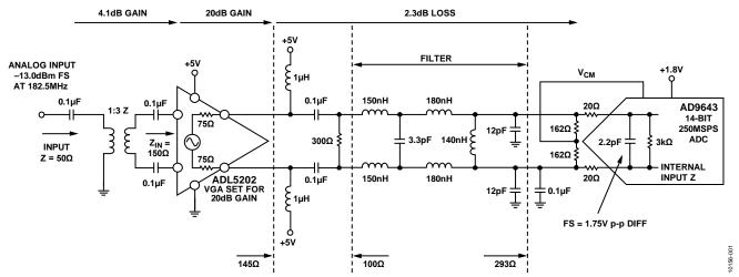
Figure 1. Single Channel of Quad IF Receiver Front End (Simplified Schematic: All Connections and Decoupling Not Shown),
