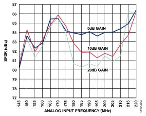
Figure 4. SFDR Performance vs. Analog Input Frequency (0 dB Gain, 10 dB Gain, and 20 dB Gain)
