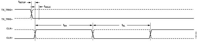
Figure 2. TX\_TRIG± to CLK± Input Timing
