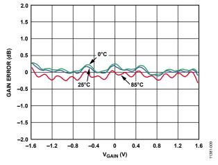
Figure 9. Gain Error vs. VGAIN
