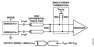
Figure 47. AC-Coupled Digital Output Termination Example
