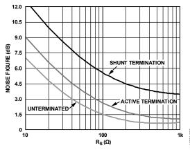
Figure 35. Noise Figure vs.  $R_S$  for Shunt Termination, Active Termination Matched and Unterminated Inputs,  $V_{GAIN} = 1.6 \text{ V}$
