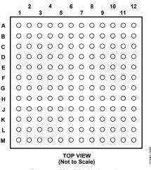
Figure 8. CSP\_BGA Pin Location
