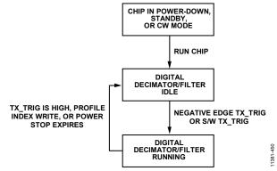
Figure 59. Digital Block Power Saving Scheme
