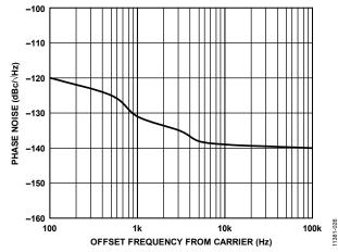
Figure 26. TGC Path Phase Noise, LNA Gain = 21.6 dB, PGA Gain = 27 dB, V<sub>GAIN</sub> = 0 V
