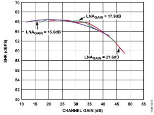
Figure 18. SNR vs. Channel Gain and LNA Gain,  $A_{OUT} = -1.0 \text{ dBFS}$
