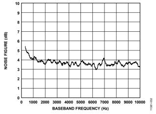
Figure 31. Noise Figure vs. Baseband Frequency
