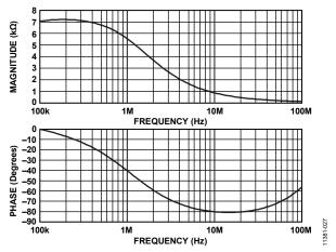
Figure 27. LNA Input Impedance Magnitude and Phase, Unterminated
