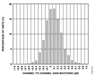
Figure 13. Gain Matching Histogram,  $V_{GAIN} = -1.2 \text{ V}$
