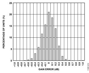
Figure 12. Gain Error Histogram, V<sub>GAIN</sub> = 1.28 V
