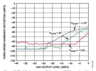
$\textit{Figure 25. Third-Order Harmonic Distortion vs. ADC Output Level (A_{OUT})}$
