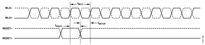
$\textit{Figure 6. CW Doppler Mode Input MLO$\pm$, Pulse Asynchronous \textit{RESET$\pm$ Timing, 4LO/8LO/16LO Mode}$
