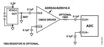
Figure 42. Single-Ended 1.8 V CMOS Sample Clock
