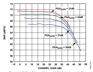
Figure 19. SNR vs. Channel Gain and PGA Gain,  $A_{\text{IN}} = -45 \text{ dBm}$
