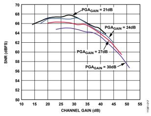
Figure 17. SNR vs. Channel Gain and PGA Gain,  $A_{OUT} = -1.0 \text{ dBFS}$
