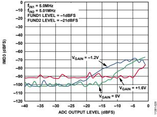
Figure 29. IMD3 vs. ADC Output Level
