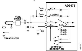
Figure 37. Simplified LNA Input Configuration
