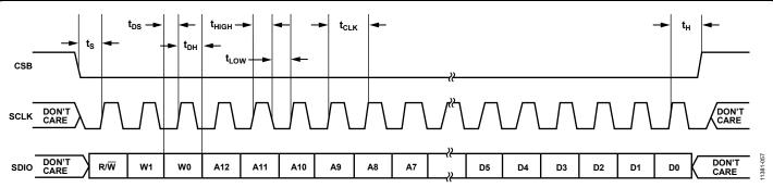
Figure 61. Serial Timing Details
