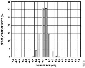
Figure 11. Gain Error Histogram, V<sub>GAIN</sub> = 0 V
