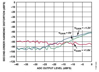
Figure 24. Second-Order Harmonic Distortion vs. ADC Output Level (A $_{\text{OUT}}$ )
