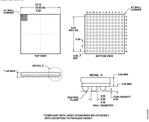
Figure 62. 144-Ball Chip Scale Package, Ball Grid Array [CSP\_BGA] (BC-144-1) Dimensions shown in millimeters
