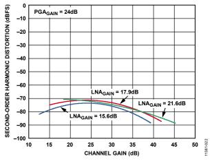
Figure 22. Second-Order Harmonic Distortion vs. Channel Gain,  $A_{OUT} = -1.0 \text{ dBFS}$
