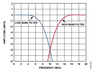
Figure 58. AAF Frequency Response, Zoomed In (Frequency Scale Assumes  $f_{ADC} = 2 \times f_{DEC} = 40 \text{ MHz}$ )
