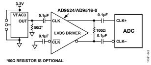
Figure 41. Differential LVDS Sample Clock
