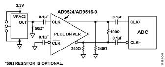
Figure 40. Differential PECL Sample Clock
