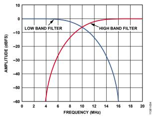
Figure 57. AAF Frequency Response (Frequency Scale Assumes  $f_{ADC} = 2 \times f_{DFC} = 40 \text{ MHz}$ )
