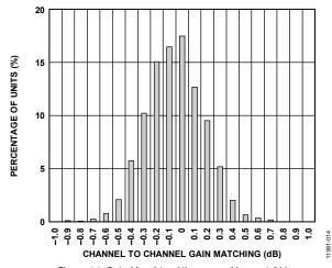
Figure 14. Gain Matching Histogram, V<sub>GAIN</sub> = 1.2 V
