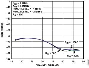
Figure 28. IMD3 vs. Channel Gain
