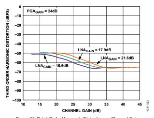
Figure 23. Third-Order Harmonic Distortion vs. Channel Gain,  $A_{OUT} = -1.0 \text{ dBFS}$
