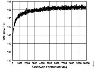
Figure 32. Output Referred SNR vs. Baseband Frequency
