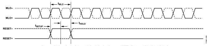
Figure 5. CW Doppler Mode Input MLO±, Pulse Synchronous RESET± Timing, 4LO/8LO/16LO Mode
