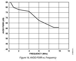
The ratio shown in Figure 16 is calculated as amps out with respect to volts in. Noise on the AVDD pin can modulate the internal switches and, therefore, modulate the output current. Therefore, the voltage noise on the AVDD pin is added in a nonlinear manner to the desired IOUTFS.
