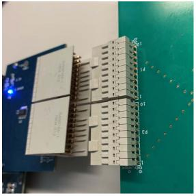
Figure 21. CMOS DAC/DPG2 Connected to AD-DAC-FMC-ADP
