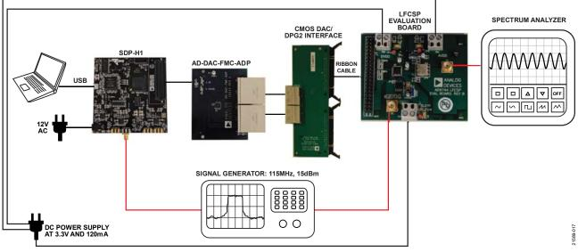
Figure 18. Hardware Connections
