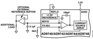
Figure 3. Internal Reference Configuration
