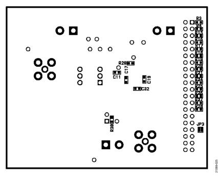
Figure 40. AD9740ACP-PCBZ/AD9742ACP-PCBZ/AD9744ACP-PCBZ/AD9748ACP-PCBZ LFCSP Evaluation Board Layout Assembly—Secondary Side
