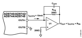
Figure 15. Unipolar Buffered Voltage Output
