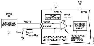
Figure 4. External Reference Configuration
