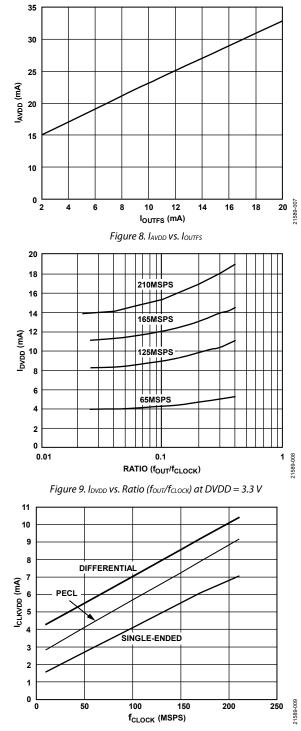
Figure 10. ICLKVDD vs. fCLOCK and Clock Mode
