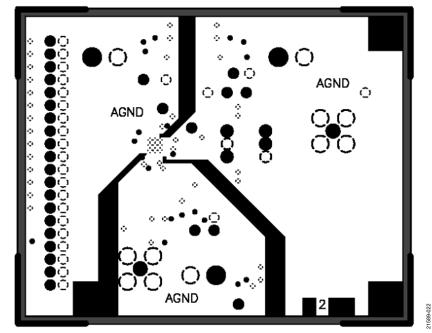
Figure 37. AD9740ACP-PCBZ/AD9742ACP-PCBZ/AD9744ACP-PCBZ/AD9748ACP-PCBZ LFCSP Evaluation Board Layout—Ground Plane
