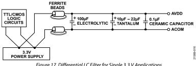
Figure 17. Differential LC Filter for Single 3.3 V Applications
