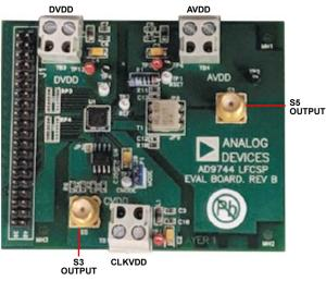
Figure 22. Evaluation Board Connectors
