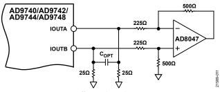
Figure 12. DC Differential Coupling Using an Op Amp
