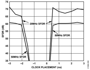
Figure 7. SFDR vs. Clock Placement at Output Frequency ( $f_{OUT}$ ) = 20 MHz and 50 MHz (Lines Connect Outside the Plot)
