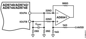
Figure 13. Single-Supply DC Differential Coupled Circuit
