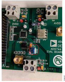
Figure 19. Evaluation Board JP1 Jumper Shunt
