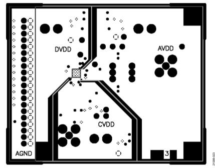
Figure 38. AD9740ACP-PCBZ/AD9742ACP-PCBZ/AD9744ACP-PCBZ/AD9748ACP-PCBZ LFCSP Evaluation Board Layout—Power Plane
