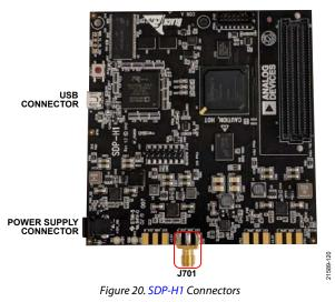
3. Connect a 12 V dc power supply to the power supply connector outlet on the SDP-H1, as shown in Figure 20.
