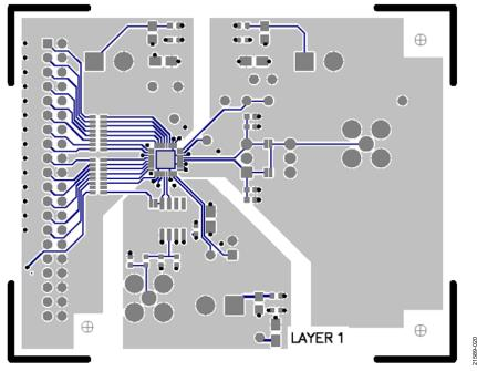
Figure 35. AD9740ACP-PCBZ/AD9742ACP-PCBZ/AD9744ACP-PCBZ/AD9748ACP-PCBZ LFCSP Evaluation Board Layout—Primary Side
