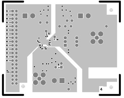
Figure 36. AD9740ACP-PCBZ/AD9742ACP-PCBZ/AD9744ACP-PCBZ/AD9748ACP-PCBZ LFCSP Evaluation Board Layout—Secondary Side
