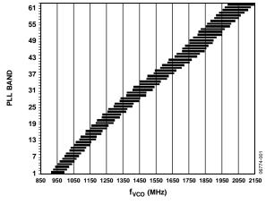
Figure 1. Typical Lock Ranges at 25℃
