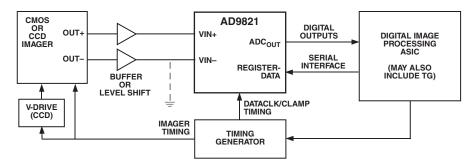
Figure 12. System Applications Diagram
