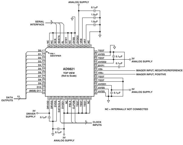
Figure 13. Recommended Circuit Configuration
