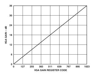
Figure 11. VGA Gain Curve
