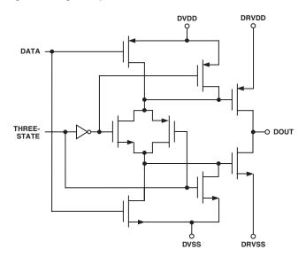
Figure 2. Data Outputs - D0-D11
