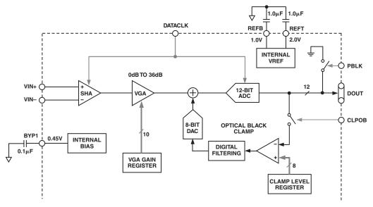
Figure 10. Internal Block Diagram
