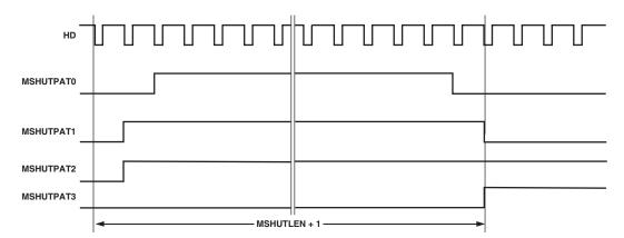
Figure 44. MSHUT Patterns Available by Setting MSHUTPAT Register
