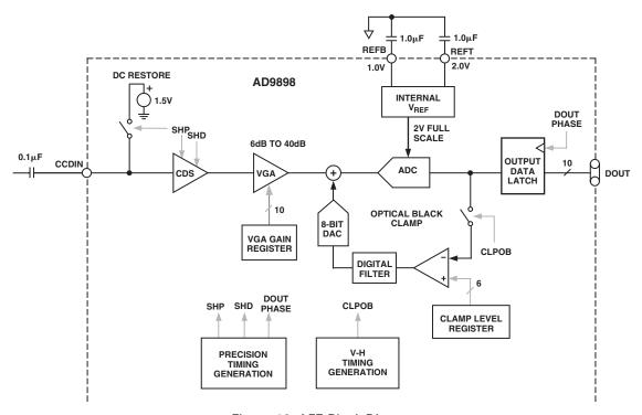
Figure 10. AFE Block Diagram
