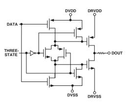
Figure 2. Digital Data Outputs
