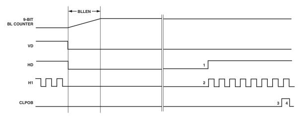
1. POSITIONS 1, 2, 3, AND 4 ARE DELAYED BY THE VALUE OF THE BL COUNTER. 2. VSG1, VSG2, V1–V4, AND SUBCK PULSES ARE NOT DELAYED BY THE BL COUNTER.
