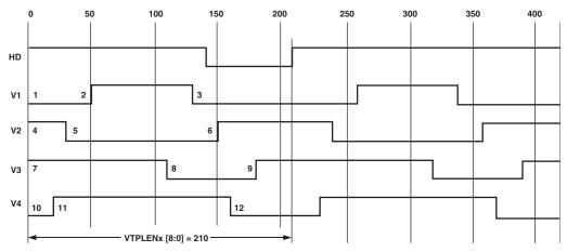
Figure 29. Step 2: Create Individual Sequences for V1–V4 Outputs by Assigning Pulse Repetitions to VTP0, VTP1, VTP2, and VTP3 Patterns. This Example Shows VTPREPx = 2.
