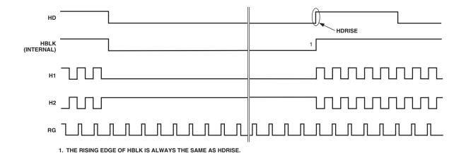
Figure 23. Normal H-Blanking Operation HBLKMASK = 0, HPULSECNT = 0, HBLKHPOS = xxx
