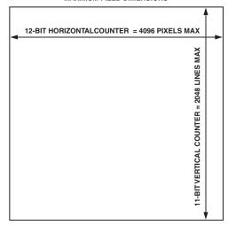
Figure 6. Horizontal and Vertical Counters
