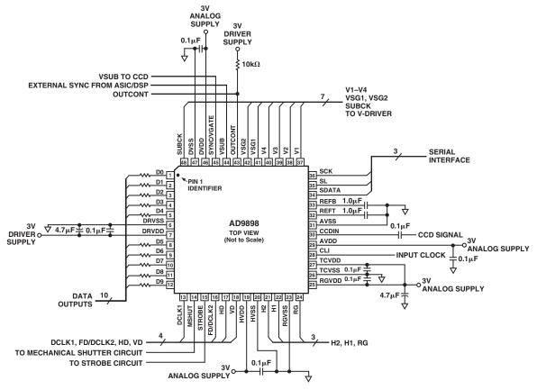
Figure 58. Typical Circuit Configuration
