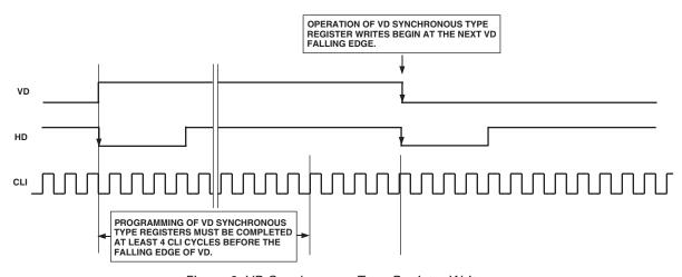
Figure 9. VD Synchronous Type Register Writes
