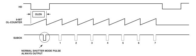
Figure 39. Electronic Shutter Timing
