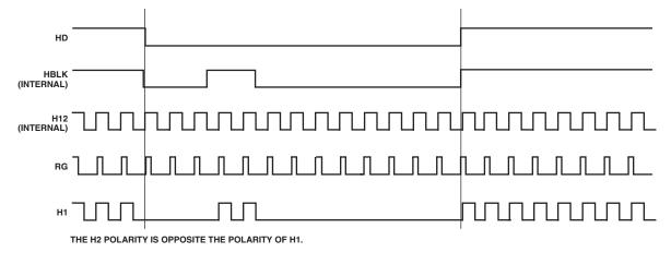
Figure 24. Selective H-Blanking Operation HBLKMASK = 0, HPULSECNT = 1, HBLKHPOS = 003
