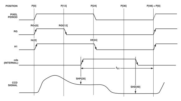
1. ALL SIGNAL EDGES ARE FULLY PROGRAMMABLETO ANY OF THE 48 POSITIONS WITHIN ONE PIXEL PERIOD. 2. DEFAULT POSITIONS FOR EACH SIGNAL ARE SHOWN.
