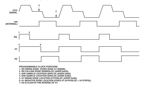
Figure 12. High Speed Clock Programmable Locations
