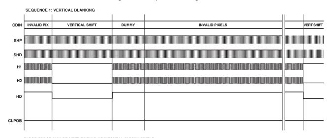
CLPOB PULSE MAY BE USED DURING HORIZONTAL DUMMY PIXELS IF THE H-CLOCKS ARE USED DURING VERTICAL BLANKING.
