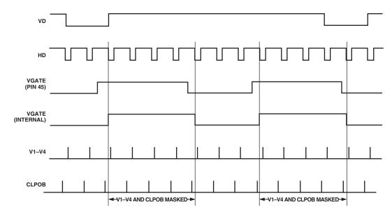
Figure 26. Example of VGATE Input Masking V1-V4 and CLPOB Outputs with MSHUT/VGATE\_EN = 0
