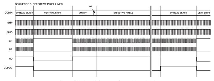
Figure 57. Horizontal Sequences during Effective Pixels
