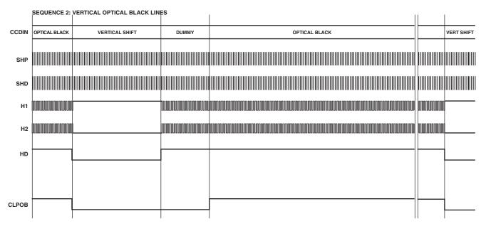
Figure 56. Horizontal Sequence during Vertical Optical Black Pixels
