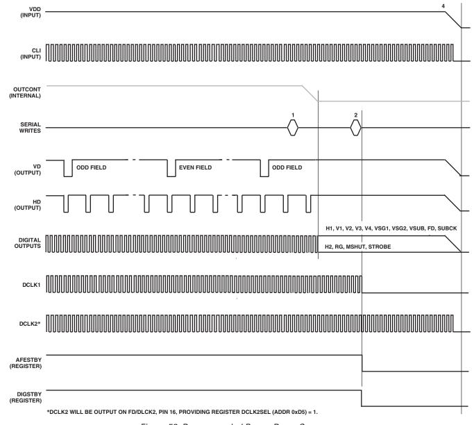
Figure 53. Recommended Power-Down Sequence
