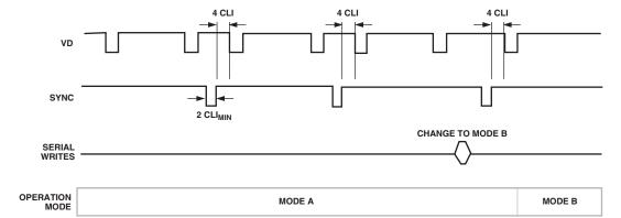
Figure 16. Example of Synchronization with SYNCPOL = 0 and SYNCCNT = 1
