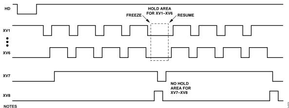
1. WHEN HOLD = 1 FOR ANY V-SEQUENCE, THE FREEZE AND RESUME REGISTERS ARE USED TO SPECIFY THE HOLD AREA BOUNDRIES. 2. WHEN XV78HOLDEN = 0, XV7 AND XV8 DO NOT USE THE HOLD AREA, ONLY XV1–XV6. H-COUNTER FOR XV1–XV6 WILL STOP DURING HOLD AREA.
