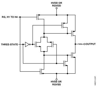
Figure 5. Digital Data Outputs
