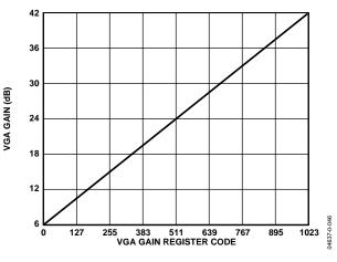
Figure 56. VGA Gain Curve
