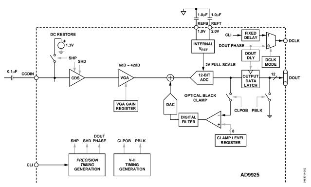
Figure 55. Analog Front End Functional Block Diagram
