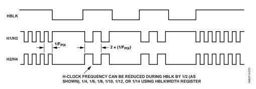
Figure 27. Generating Wide H-Clock Pulses during HBLK Interval
