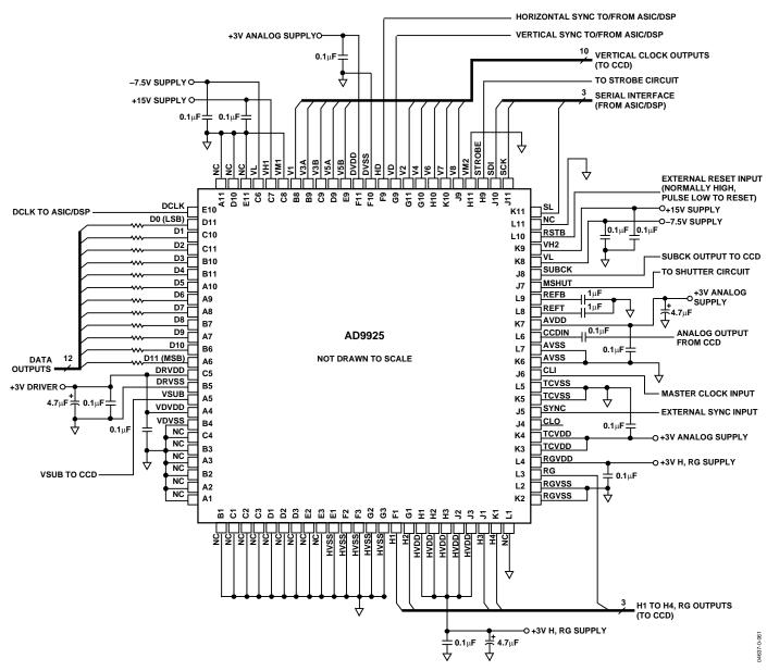
Figure 73. AD9925 Typical Circuit Configuration
