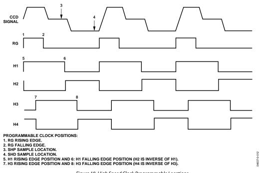
Figure 18. High Speed Clock Programmable Locations
