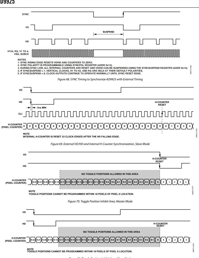
Figure 71. Toggle Position Inhibit Area, Slave Mode
