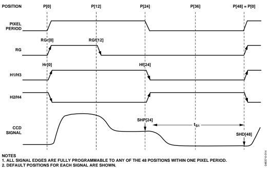
Figure 20. High Speed Timing Default Locations
