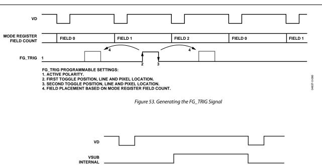
Figure 54. Combining FG\_TRIG and VSUB to Create Four Toggle Positions for VSUB Output
