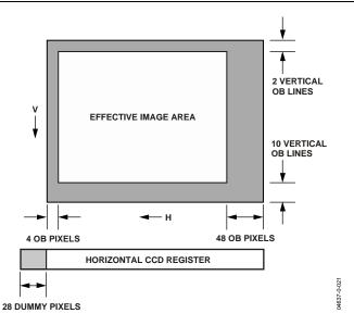
Figure 28. Example CCD Configuration
