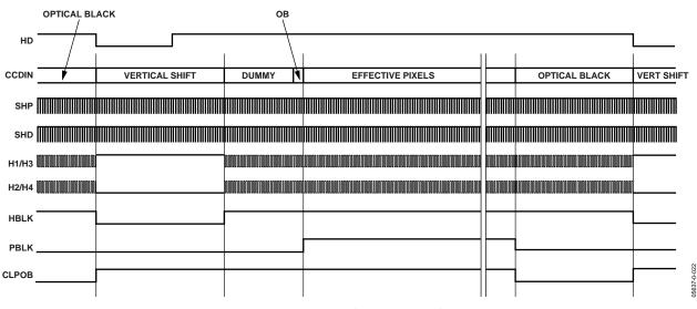
Figure 29. Horizontal Sequence Example
