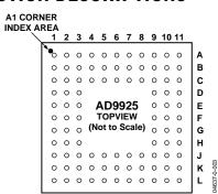
Figure 3. 96-Lead CSPBGA Package Pin Configuration
