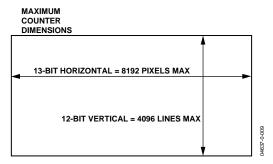
Figure 15. Vertical and Horizontal Counters
