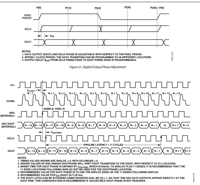
*Figure 22. Digital Data Output Pipeline Delay*
