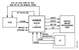
Figure 14. Typical System Block Diagram, Master Mode
