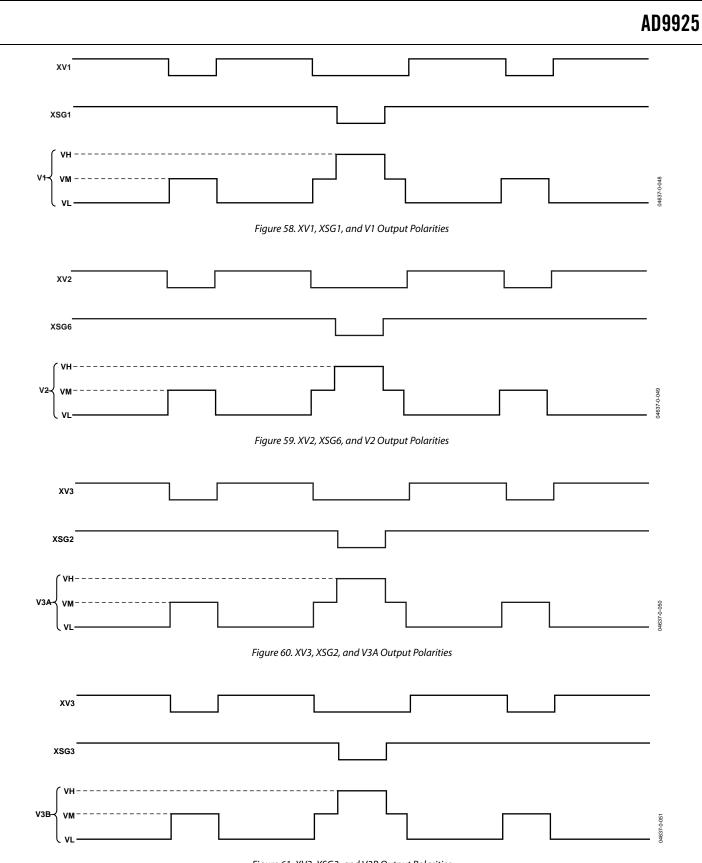
Figure 61. XV3, XSG3, and V3B Output Polarities
