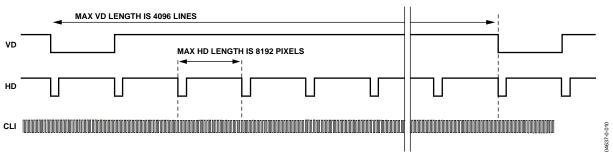
Figure 16. Maximum VD/HD Dimensions
