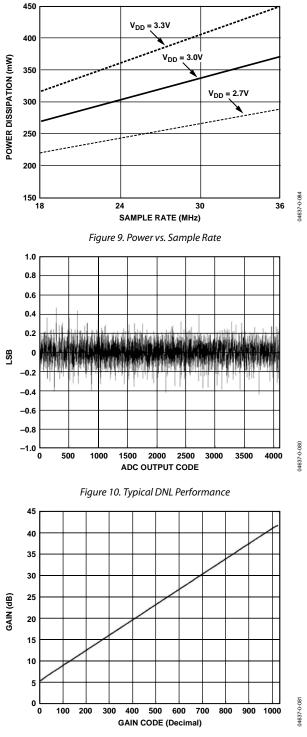
Figure 11. Typical VGA Gain Curve
