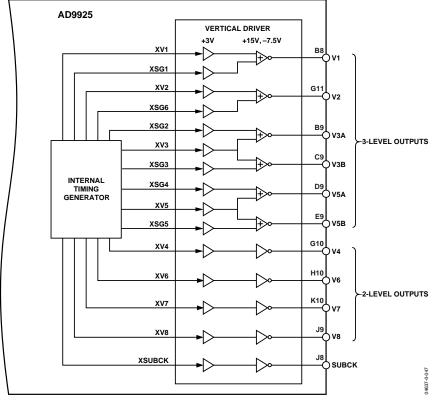
Figure 57. AD9925 Internal V-Driver Input Signals
