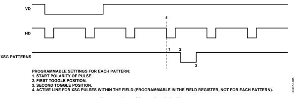
Figure 42. Vertical Sensor Gate Pulse Placement
