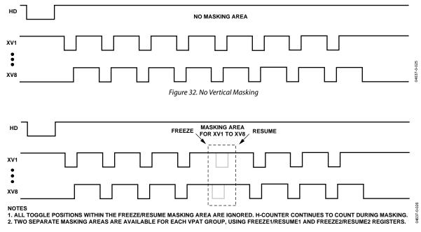
Figure 33. Vertical Masking Using the FREEZE/RESUME Registers
