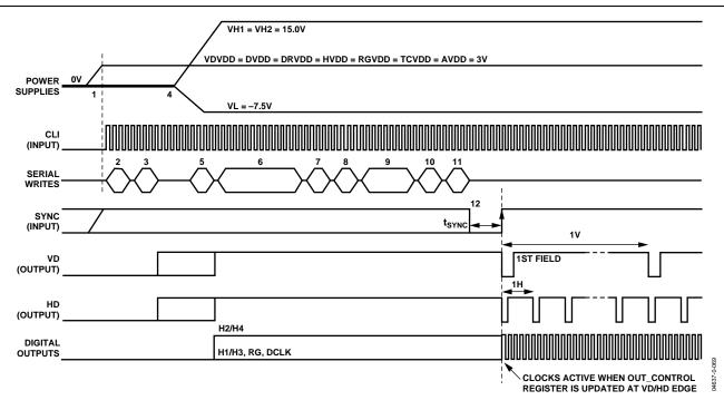
Figure 67. Recommended Power-Up Sequence and Synchronization, Master Mode
