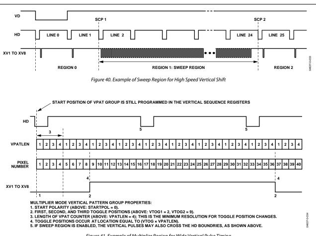
Figure 41. Example of Multiplier Region for Wide Vertical Pulse Timing
