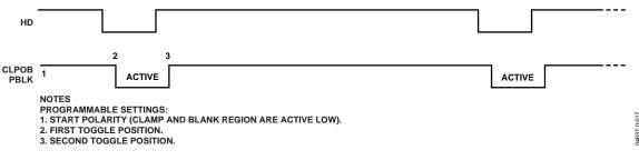
Figure 23. Clamp and Preblank Pulse Placement
