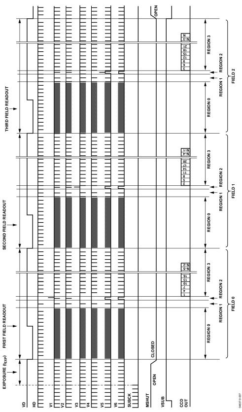
Figure 44. CCD Timing Example—Dividing Each Field into Regions
