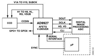
Figure 13. Typical System Block Diagram, Master Mode
