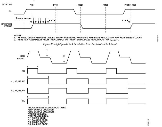
Figure 17. High Speed Clock Programmable Locations (HCLKMODE = 001)
