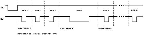
SPC\_PAT\_EN[0] = 1 VREPA = N V-PATTERN B IS USED AS SPECIAL PATTERN TOTAL NUMBER OF REPS USED FOR SEQUENCE (N REPS) VREPB = 4 REP 4 USES V-PATTERN B INSTEAD OF V-PATTERN A
