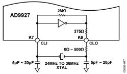
Figure 96. Crystal Application Using CLI/CLO (Consult Crystal Data Sheet for Component Values)
