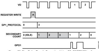
$\textit{Figure 75. ShotDelay Toggle Operation Using GP\_PROTOCOL} = 3$
