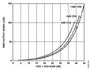
Figure 6. Output Noise vs. Total Gain (CDS + VGA)
