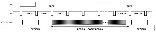
Figure 50. Example of Sweep Region for High Speed Vertical Shift
