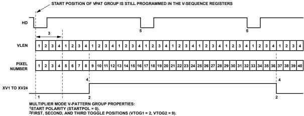
3LENGTH OF VPAT COUNTER (VLEN = 4); THIS IS THE MINIMUM RESOLUTION FOR TOGGLE POSITION CHANGES. 4TOGGLE POSITIONS OCCUR AT LOCATION EQUAL TO (VTOG × VLEN).
