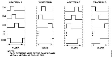
Figure 40. Vertical Timing Divided Into Four Segments: VPATA, VPATB, VPATC, and VPATD
