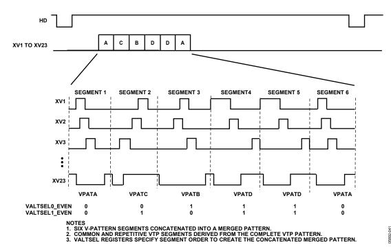
Figure 42. Example of Special V-Sequence Alternation Mode Using VALTSEL Registers to Specify Segment Order
