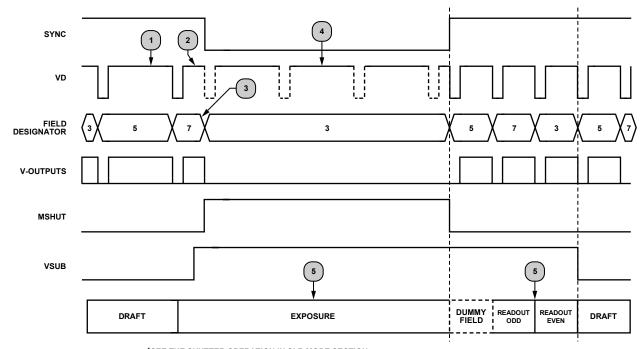
Figure 84. Enhanced SYNC Mode—Manual Shutter Operation, SLR Mode
