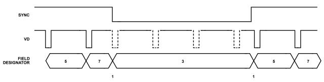
Figure 83. Special SYNC Mode Effect on Field Designator
