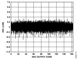
Figure 5. Typical Differential Nonlinearity (DNL) Performance
