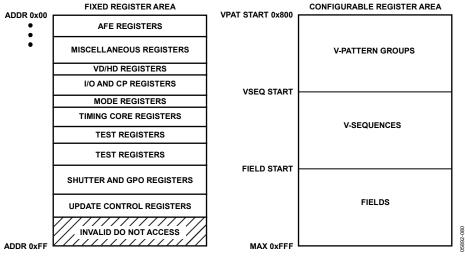
Figure 99. Layout of AD9927 Registers
