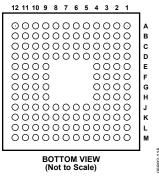
Figure 3. Pin Configuration
