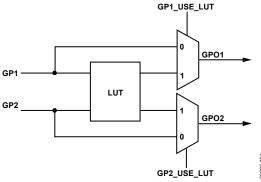
Figure 76. Internal LUT for GP1 and GP2 Signals
