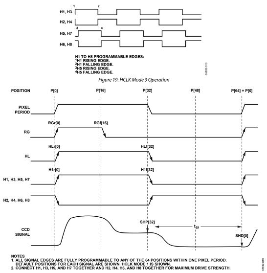
Figure 20. High Speed Timing Default Locations
