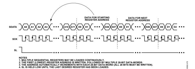
Figure 98. Continuous Serial Write Operation
