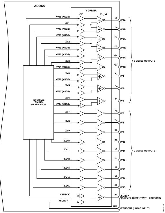
Figure 53. Internal AFETG to V-Driver Connections
