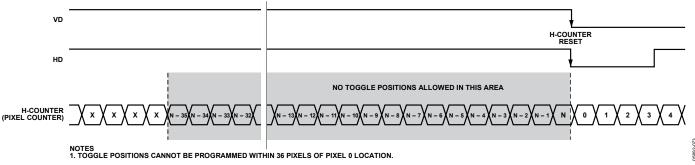
Figure 91. Toggle Position Inhibited Area—Master Mode
