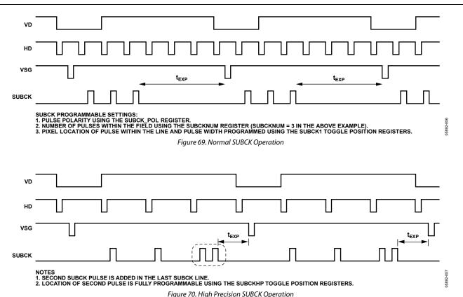
Figure 70. High Precision SUBCK Operation
