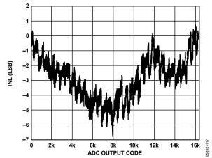
Figure 7. Typical System Nonlinearity Performance
