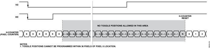
Figure 92. Toggle Position Inhibited Area—Slave Mode
