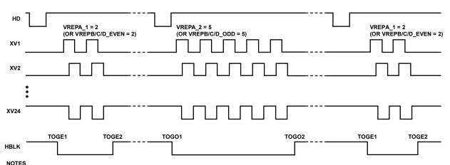
Figure 43. Odd/Even Line Alternation of V-Pattern Group Repetitions and HBLK Toggle Positions
