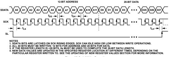
Figure 97. Serial Write Operation
