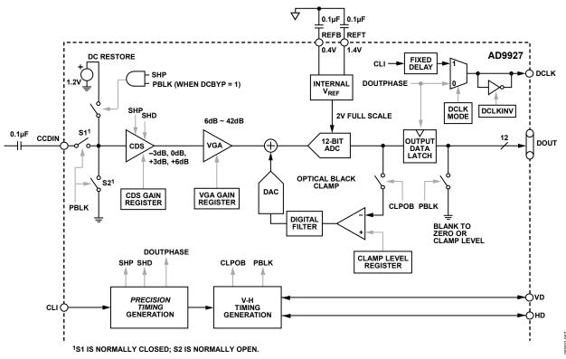
Figure 85. Analog Front-End Functional Block Diagram
