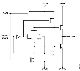
Figure 9. Digital Data Outputs
