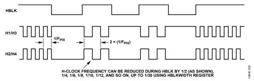
Figure 29. Generating Wide H-Clock Pulses During HBLK Interval
