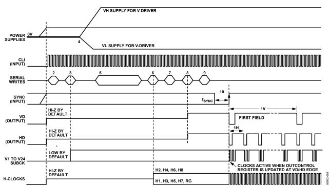
Figure 87. Recommended Power-Up Sequence and Synchronization, Master Mode
