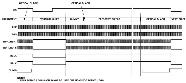
Figure 33. Horizontal Sequence Example
