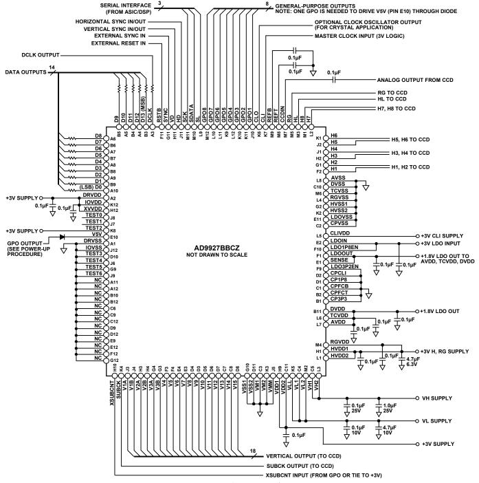
Figure 94. Typical 3 V Circuit Configuration
