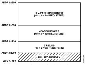
Figure 100. Example Register Configuration
