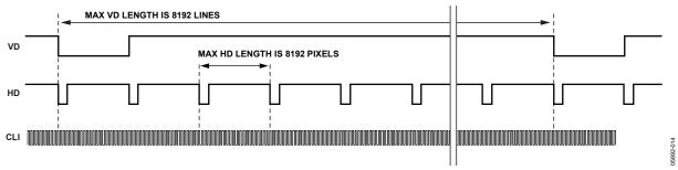
Figure 15. Maximum VD/HD Dimensions
