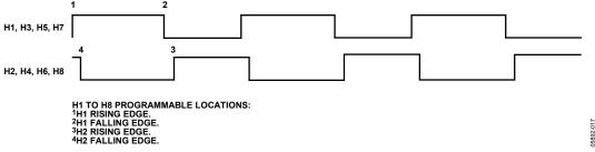
Figure 18. HCLK Mode 2 Operation
