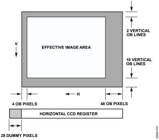
Figure 32. Example CCD Configuration
