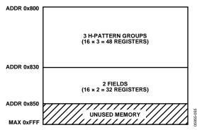
Figure 55. Example Register Configuration
