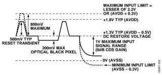
Figure 2. Input Signal Characteristics
