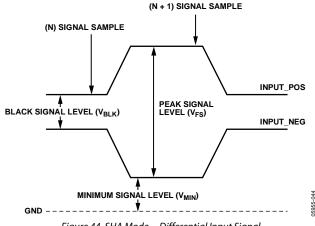
Figure 44. SHA Mode—Differential Input Signal
