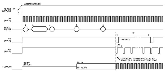
Figure 48. Recommended Power-Up Sequence
