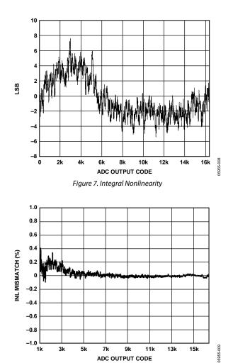
ADC OUTPUT CODE Figure 8. Linearity Mismatch vs. ADC Output Code
