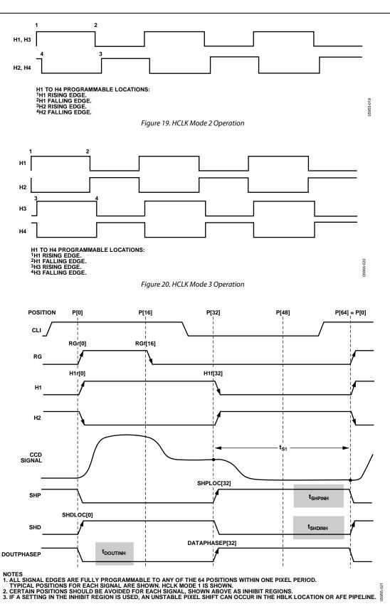
Figure 21. High Speed Timing Default Locations
