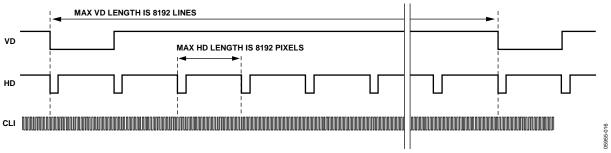
Figure 16. Maximum VD/HD Dimensions
