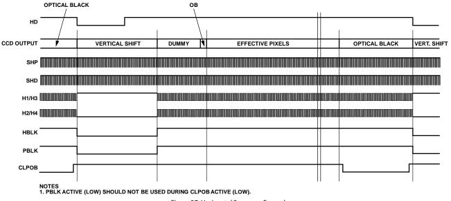
Figure 37. Horizontal Sequence Example
