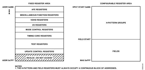
Figure 54. Layout of AD9974 Registers
