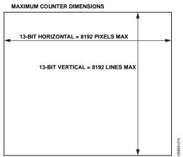
Figure 15. Vertical and Horizontal Counters
