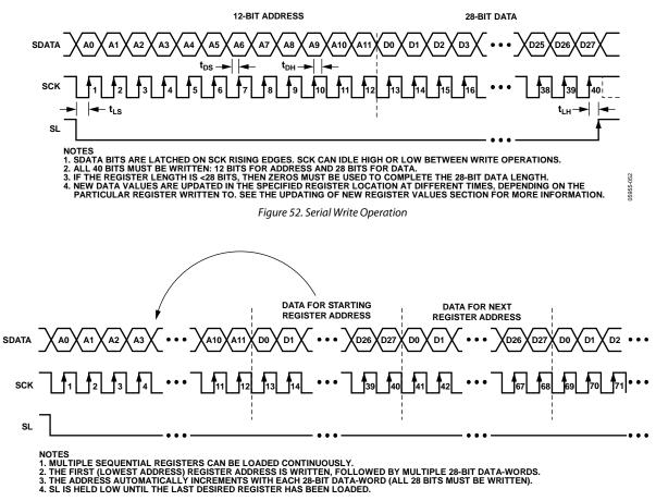
Figure 53. Continuous Serial Write Operation
