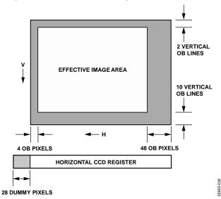
Figure 36. Example CCD Configuration
