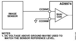
Figure 45. SHA Mode—Single–Ended Input Configuration, DC-Coupled
