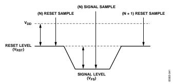
Figure 41. Traditional Inverting CDS Signal
