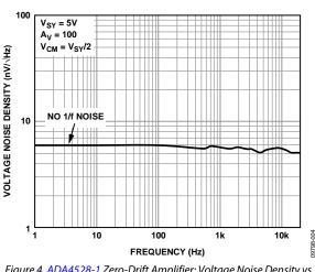
Figure 4. ADA4528-1 Zero-Drift Amplifier: Voltage Noise Density vs. Frequency
