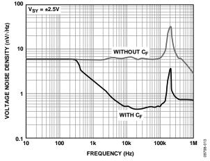
Figure 10. Voltage Noise Density with Feedback Capacitor
