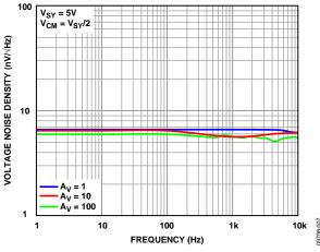
Figure 6. ADA4528-1: Voltage Noise Density vs. Frequency
