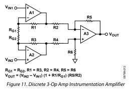
To build a discrete instrumentation amplifier with external resistors without compromising on noise, pay close attention to the resistor values chosen.  $R_{G1}$  and  $R_{G2}$  each has thermal noise that is amplified by the total noise gain of the instrumentation amplifier and, therefore, should be chosen sufficiently low to
