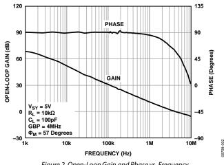
Figure 2. Open-Loop Gain and Phase vs. Frequency
