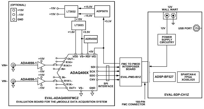
Figure 2. Simplified Evaluation Board Block Diagram
