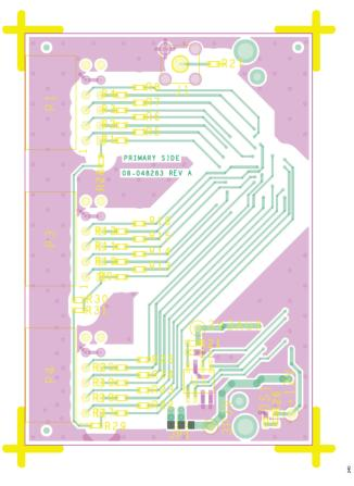
Figure 33. EVAL-PMD-IB1Z, Top Layer
