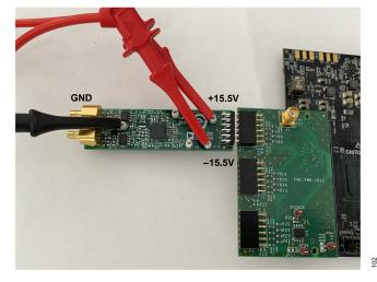
Figure 3. EVAL-ADAQ4001PMDZ and EVAL-ADAQ4003PMDZ External Supply (Optional) Connections
