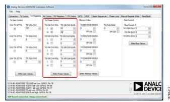
Figure 12. Setting Transmit Channel 1 to 45° in Transmit Phase Control with All Other Channels at 0°
