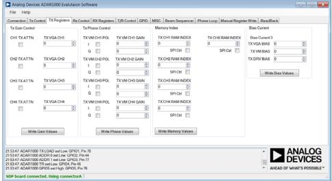
Figure 29. TX Registers Tab
