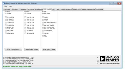
Figure 32. T/R Control Tab
