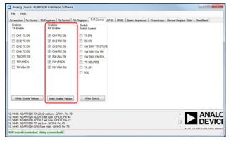
Figure 15. Enabling Receive Channels
