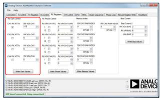
Figure 18. Setting Receive Channel 1 to Maximum Gain in Receive Gain Control with All Other Channels at Minimum Gain
