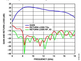
Figure 26. Transmit Mode Gain and Return Loss
