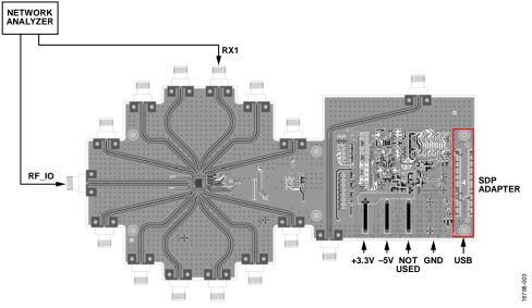
Figure 3. Typical Evaluation Board Setup
