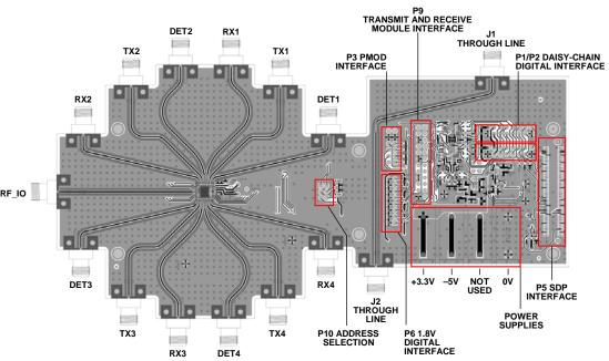
Figure 2. ADAR1000-EVALZ Evaluation Board Connections
