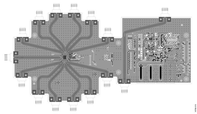
Figure 41. Layer 1 (Component Side)
