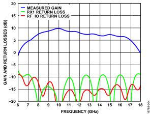
Figure 25. Receive Mode Gain and Return Loss Measurement Results
