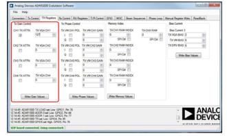
Figure 11. Setting Transmit Channel 1 to Maximum Gain in Transmit Gain Control with All Other Channels at Minimum Gain
