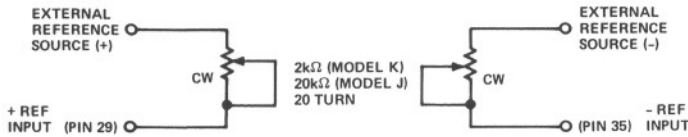
Figure 8. External Reference Connections
