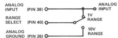
Figure 4. Range Selection Circuit
