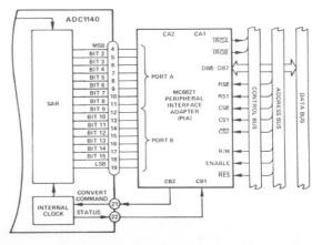
Figure 8. ADC1140 Interface to PIA
