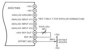
Figure 3. Offset and Gain Calibration
