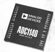
**GENERAL DESCRIPTION** The ADC1140 is a low cost 10-bit successive approximation analog-to-digital converter having a  $35\mu$ s maximum conversion time. This converter provides high accuracy, high stability and low power consumption all in a  $2'' \times 2'' \times 0.4''$  module.
