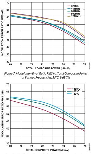
Figure 8. Modulation Error Ratio RMS vs. Total Composite Power at Various Temperatures, 57 MHz, 9 dB Tilt
