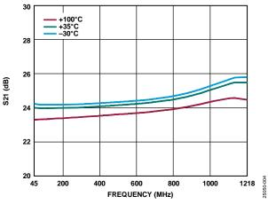
Figure 4. S21 vs. Frequency at Various Temperatures
