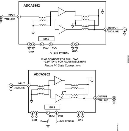
Figure 15. IADJ Bias Control Connections
