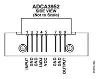
Figure 2. Pin Configuration
