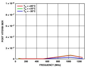
Figure 8. Post Viterbi Bit Error Rate (BER) vs. Frequency at Various Temperatures,  $V_0 = 61$  dBmV at 1218 MHz, 23 dB Extrapolated Tilt, 190 Digital Channels, Total Composite Power = 76.8 dBmV, 10 sec Integration Time
