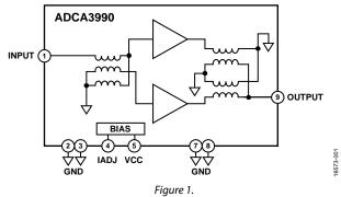
transistor (pHEMT) die and gallium nitride (GaN) HEMT die. The dc current and supply voltage can be adjusted externally for optimum distortion performance vs. power consumption over a range of output levels.
