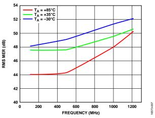
Figure 7. RMS Modulation Error Rate (MER) vs. Frequency at Various Temperatures,  $V_0 = 61 \text{ dBmV}$  at 1218 MHz, 23 dB Extrapolated Tilt, 190 Digital Channels, Total Composite Power = 76.8 dBmV
