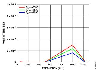
Figure 8. Post Viterbi Bit Error Rate (BER) vs. Frequency at Various Temperatures,  $V_0 = 61$  dBmV at 1218 MHz, 23 dB Extrapolated Tilt, 190 Digital Channels, Total Composite Power = 76.8 dBmV, 10 sec Integration Time
