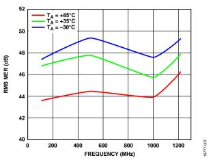
Figure 7. RMS Modulation Error Rate (MER) vs. Frequency at Various Temperatures,  $V_0 = 61$  dBmV at 1218 MHz, 23 dB Extrapolated Tilt, 190 Digital Channels, Total Composite Power = 76.8 dBmV
