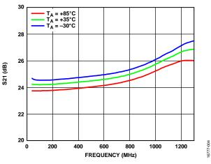
Figure 4. Gain (S21) vs. Frequency at Various Temperatures
