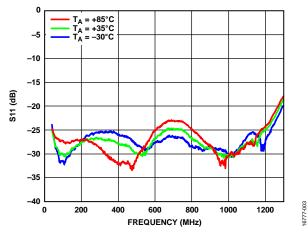
Figure 3. Input Return Loss (S11) vs. Frequency at Various Temperatures
