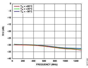
Figure 5. Reverse Isolation (S12) vs. Frequency at Various Temperatures
