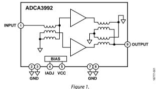
high electron mobility transistor (pHEMT) die in combination with a gallium nitride (GaN) HEMT die. The dc current and supply voltage can be adjusted externally for optimum distortion performance vs. power consumption over a range of output levels. The ADCA3992 is packaged in the industry-standard SOT115J package.
