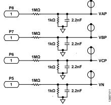
Figure 12. Final Representation of Voltage Channel Configuration
