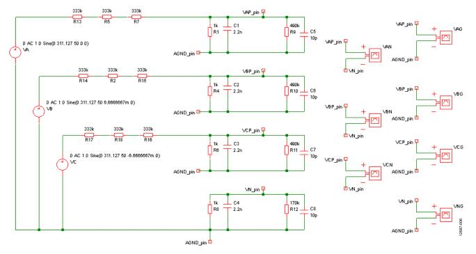
Figure 7. Simulation Test Bench: Standard 3P4W Wye Setup
