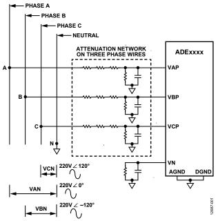
Figure 1. Standard 3P4W Wye Configuration Voltage Connection
