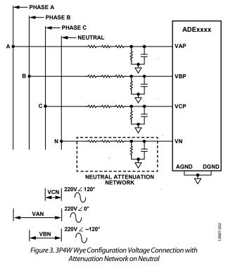
Another common alternative to remain isolated from the high voltages is the use of voltage transformers; however, voltage transformers are less preferable because they make the meter design expensive and large.
