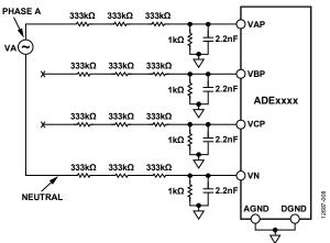
Figure 9. Phase B and Phase C Disconnected, Case 1
