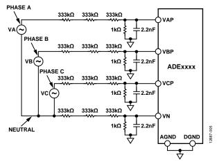
Figure 6. 3P4W Wye System: Neutral Series Resistance
