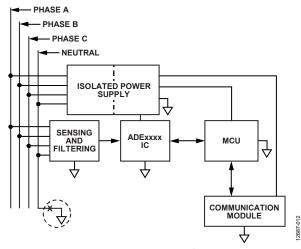
Figure 2. 3P4W Metering System Isolation Requirement
