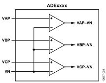
Figure 4. Voltage Channel ADC Configuration in 3-Phase ADExxxx IC
