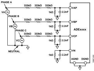
Figure 5. 3P4W Wye System: Neutral Connected to Ground
