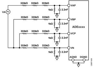
Figure 10. Phase B and Phase C Tied to Neutral, Case 2
