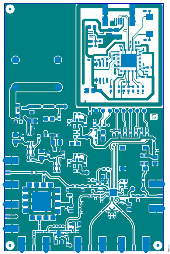
Figure 11. Layer 1 (Component Side)
