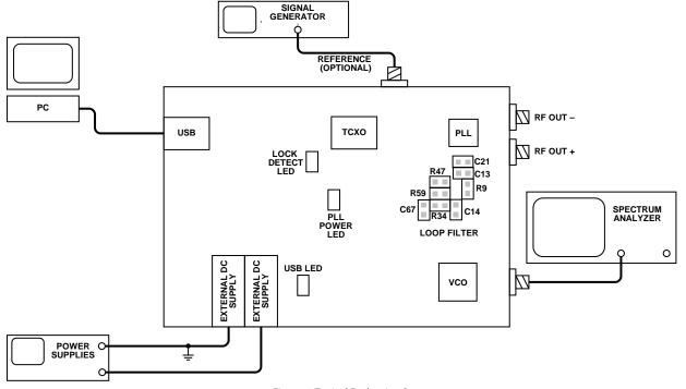
Figure 6. Typical Evaluation Setup
