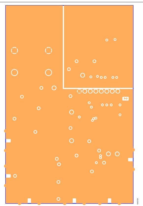
Figure 12. Layer 2 (Ground Plane)
