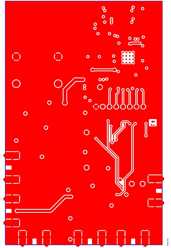
Figure 14. Layer 4 (Solder Side)
