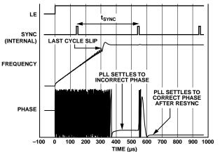
Figure 28. Phase Resync Example
