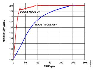
Figure 7. PLL Lock Time with Boost Mode On and Off; Locking over Octave Range Jump (1 GHz to 2 GHz) for PFD = 20 MHz, Loop Bandwidth = 100 kHz,  $I_{CP} = 300 \,\mu\text{A}, \, V_P = 28 \, V, \, AV_{DD} = DV_{DD} = SDV_{DD} = 3.3 \, V, \, REF_{IN} = 100 \, MHz$
