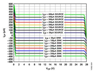
Figure 5. Charge Pump Output Characteristics,  $V_P$  = 28 V,  $I_{CP}$  Varied from 50  $\mu$ A to 400  $\mu$ A,  $R_{SET}$  = 5.1  $k\Omega$
