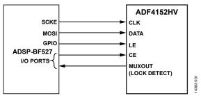
Figure 33. ADSP-BF527 to ADF4152HV Interface
