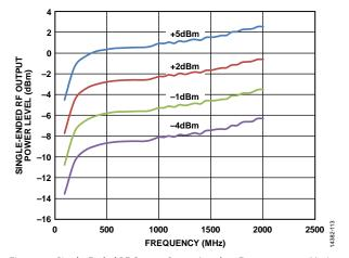
Figure 14. Single-Ended RF Output Power Level vs. Frequency over Various Power Settings, RF Output Pins Pulled Up to 3.3 V via 27 nH $\parallel$ 50  $\Omega$
