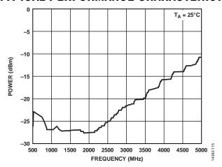
Figure 4. RF Input Sensitivity, RF Output Disabled
