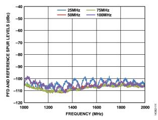
Figure 12. PFD and Reference Spur Levels vs. Frequency, Measured at VCO Output with ADL5541 Buffer Placed Between VCO Output and RF Input, REF $_{\rm IN}$  = 100 MHz, PFD = 25 MHz
