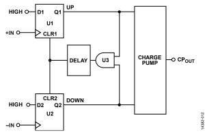
Figure 17. PFD Simplified Schematic
