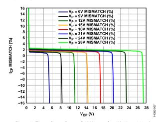
Figure 8. Charge Pump Output ( $I_{CP}$ ) Mismatch vs.  $V_{CP}$ ,  $I_{CP} = 200 \,\mu\text{A}$
