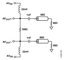
Figure 35. Optimum ADF4152HV Output Stage
