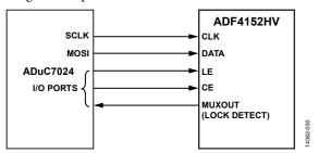
Figure 32. ADuC7024 to ADF4152HV Interface
