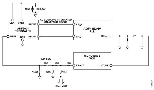
Figure 30. 16 GHz Microwave PLL
