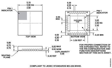
Figure 36. 32-Lead Lead Frame Chip Scale Package [LFCSP] 5 mm × 5 mm Body and 0.75 mm Package Height (CP-32-11) Dimensions shown in millimeters
