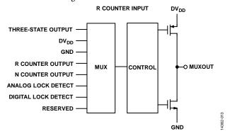
Figure 18. MUXOUT Schematic
