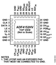
Figure 3. Pin Configuration
