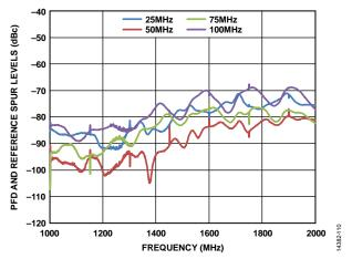
Figure 11. PFD and Reference Spur Levels vs. Frequency, Measured at VCO Output,  $REF_{IN} = 100 \text{ MHz}$ , PFD = 25 MHz
