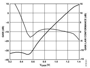
Figure 23. Power Gain Range for –10 dBm Out of the IQ Modulator, and Gain Law Conformance vs. V<sub>GAIN</sub> at 2350 MHz
