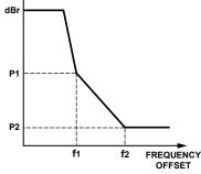
Figure 10. BTS WiBro Spectral Mask (RBW = 100 kHz)
