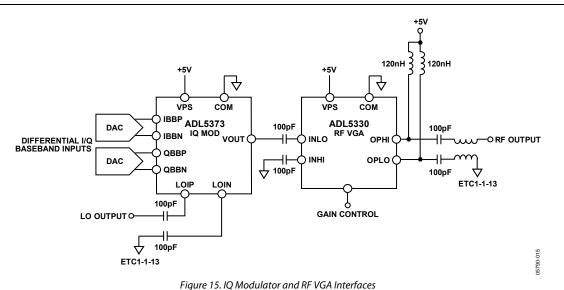
The ADL5373 is designed to drive a 50  $\Omega$  load and easily interfaces with the VGA.
