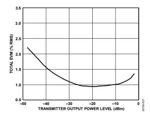
Figure 27. Transmitter Total EVM for an 802.16 64 QAM OFDM Signal, 10 MHz Signal Bandwidth
