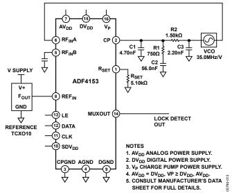
Figure 13. PLL Loop Schematic
