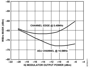
Figure 11. Modulator Performance According to WiBro Mask, with 16 QAM OFDM Modulation, Function of I and Q Input Voltage (or IQ Modulator Output Power), at 2400 MHz
