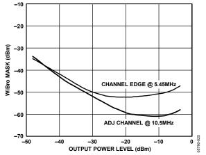
Figure 25. Transmitter Spectral Quality According to WiBro Mask (64 QAM WiMAX OFDM, 10 MHz BW) Function of Output Power or V<sub>GAIN</sub> Voltage
