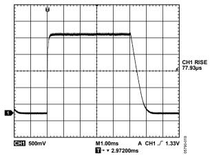
Figure 18. Power Detector Time Response to a WiMAX Downlink Burst ( $T_{SYMB} = 25.6 \ \mu s$ ), CLPF = 47 nF
