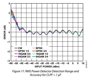
With VTG = 0.625 V (connecting VREF to VTG through a resistive divider) and a smaller CFLT capacitor, similar performances can be achieved with a fast averaging ADC. In such configuration, the RMS detector is completely insensitive to the type of OFDM modulation applied to it. Therefore, no calibration is required, whether a QPSK or a 64 QAM modulates the OFDM subcarriers. Figure 18 shows the power detector settling time for CLPF = 47 nF.
