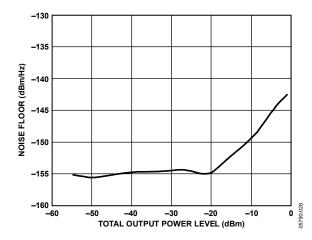
Figure 28. Transmitter Output Noise Floor vs. Output Power (QPSK, 16 QAM, 64 QAM OFDM Modulated Signal)
