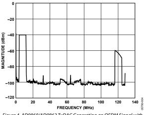
Figure 4. AD9860/AD9862 TxDAC Generating an OFDM Signal with 4× Interpolation (f<sub>SAMPLE</sub> = 32 MSPS, 4× Interpolation)
