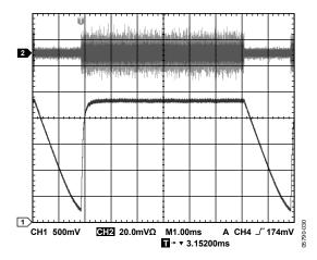
Figure 30. Power Detector Time Response for a WiMAX Downlink Burst (Long Preamble, FCH, 64 QAM OFDM Data Sequence),  $T_{SYMB} = 25.6 \ \mu s$
