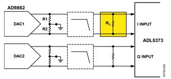
Figure 5. DAC to IQ Modulator Interface
