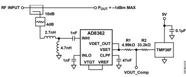
Figure 19. Power Detection and Temperature Compensation of the AD8362 at 2.35 GHz
