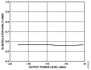
Figure 21. IQ Modulator EVM in %rms vs. Output Power, 64 QAM OFDM
