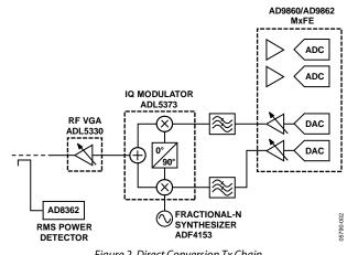
Figure 2. Direct Conversion Tx Chain
