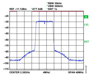
Figure 26. Transmitter Output Spectrum @ 2.35 GHz (64 QAM WiMAX OFDM, Bandwidth = 10 MHz) at -5 dBm Output Power
