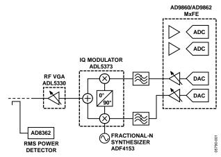
Figure 1. Direct Conversion Transmitter
