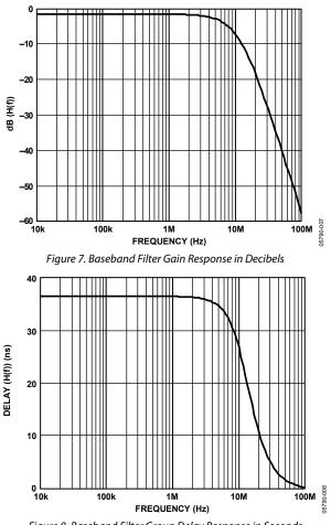
Figure 8. Baseband Filter Group Delay Response in Seconds
