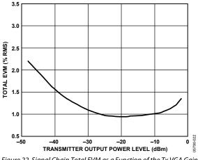
Figure 22. Signal Chain Total EVM as a Function of the Tx VGA Gain
