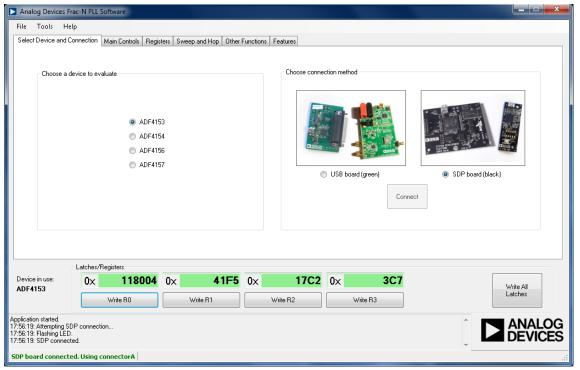
Figure 3. Software Front Panel Display—Select Device and Connection
