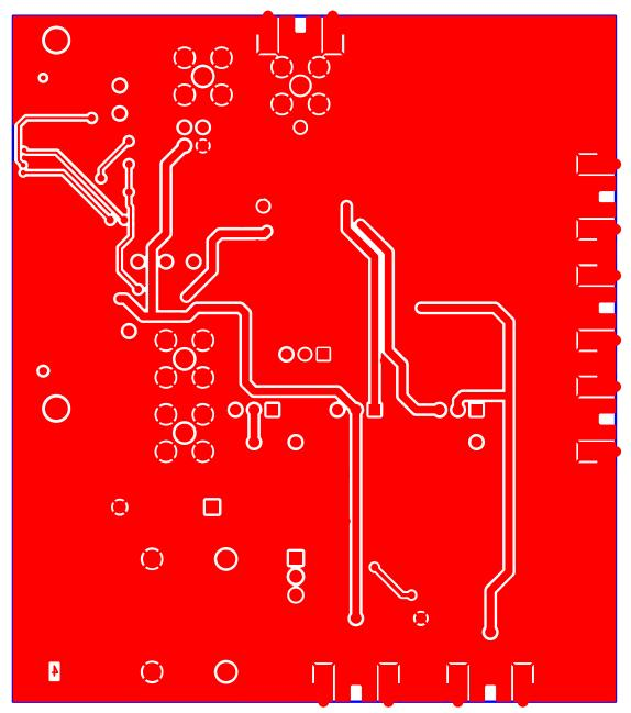
Figure 13. Layer 4 (Solder Side)
