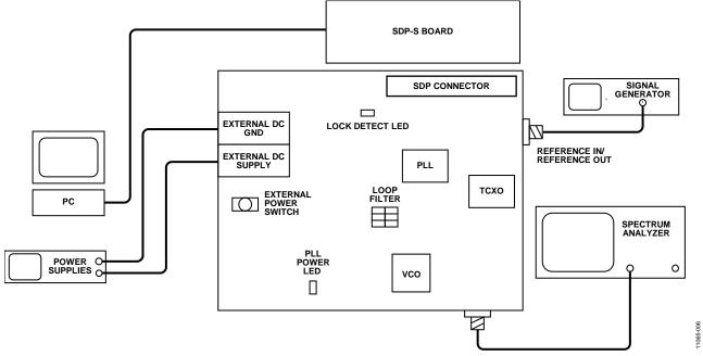
Figure 6. Typical Evaluation Setup
