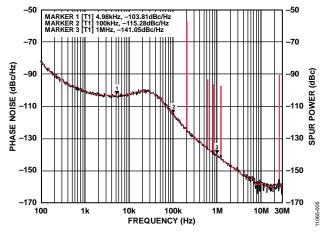
Figure 5. Spectrum Analyzer Display
