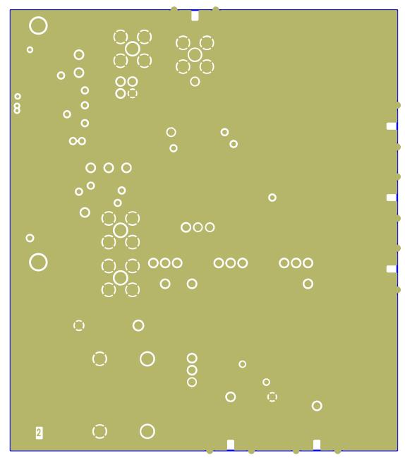
Figure 11. Layer 2 (Ground Plane)
