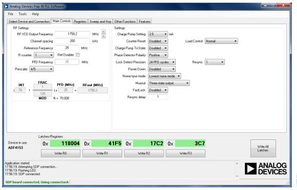
Figure 4. Software Front Panel Display—Main Controls
