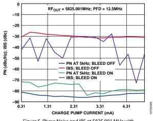
Figure 5. Phase Noise and IBS at 5825.001 MHz with a PFD Frequency = 12.5 MHz
