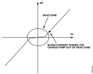
Figure 1. The Effect of Bleed Current on Charge Pump
