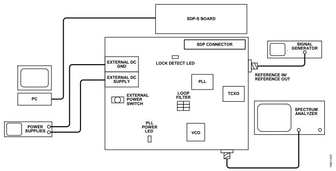
Figure 20. Typical Evaluation Setup
