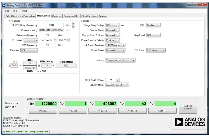
Figure 18. Frac-N PLL Software, Main Window—Main Controls
