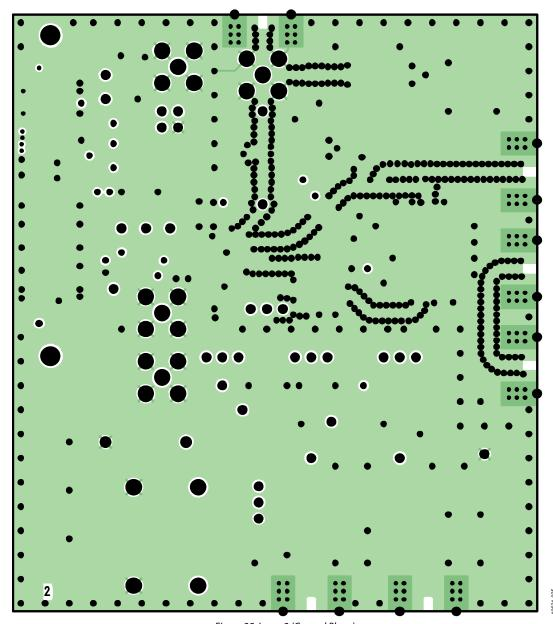
Figure 25. Layer 2 (Ground Plane)
