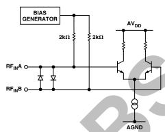
Figure 3. IF/RF Input Stage
