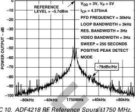
TPC 10. ADF4218 RF Reference Spurs (1750 MHz, 30 kHz, 3 kHz)
