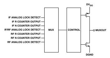
Figure 6. MUXOUT Circuit
