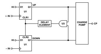
Figure 5. PFD Simplified Schematic
