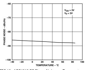
TPC 12. ADF4218 RF Phase Noise vs. Temperature (900 MHz, 200 kHz, 20 kHz)
