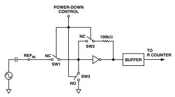
Figure 2. Reference Input Stage
