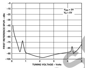
TPC 14. ADF4218 RF Reference Spurs vs.  $V_{TUNE}$  (900 MHz, 200 kHz, 20 kHz)
