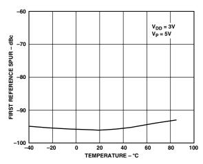
TPC 13. ADF4218 RF Reference Spurs vs. Temperature (900 MHz, 200 kHz, 20 kHz)
