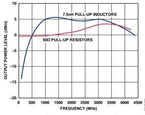
Figure 2. Comparison of the Power Level at the Output of the ADF4351 with Resistive and Inductive Pull-up Networks
