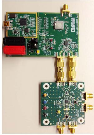
Figure 7. Board Setup Used to Interface the ADF4351 with the ADL5801
