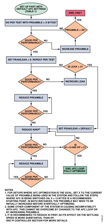
Figure 7. Recommended Steps to Find Optimum AFC Settings
