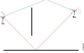
Figure 3. Multipath Propagation
