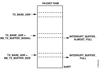
Figure 22. Rolling Buffer in Transmit Mode
