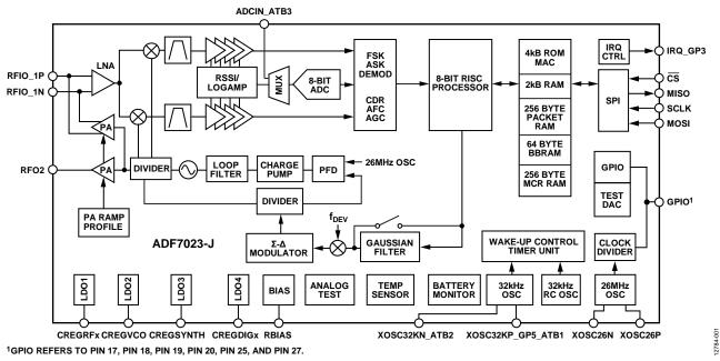
Figure 1. ADF7023-J Block Diagram
