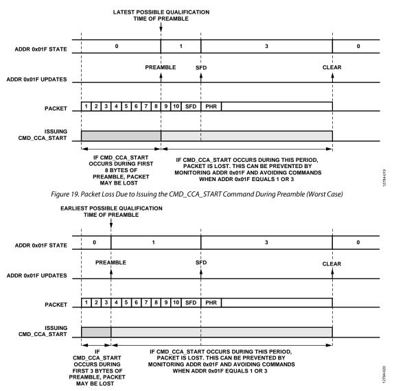
Figure 20. Packet Loss Due to Issuing the CMD\_CCA\_START Command During Preamble (Best Case)
