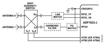
Figure 4. Typical Antenna Diversity Hardware
