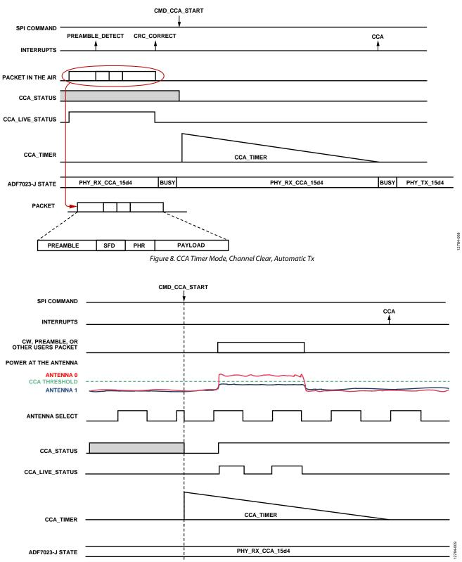
Figure 9. CCA Timer Mode, Antenna Diversity Enabled, Channel Busy
