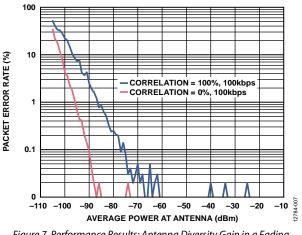
Figure 7. Performance Results: Antenna Diversity Gain in a Fading Environment
