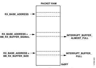
Figure 23. Rolling Buffer in Receive Mode
