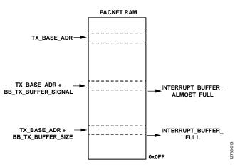
Figure 13. Rolling Buffer in Transmit Mode
