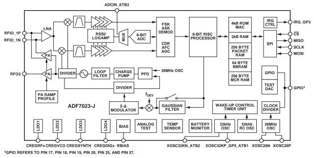
Figure 1. ADF7023-J Block Diagram
