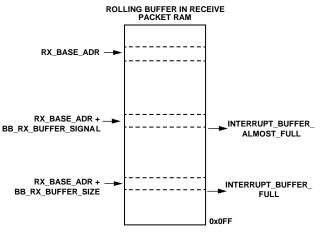
Figure 14. Rolling Buffer in Receive Mode
