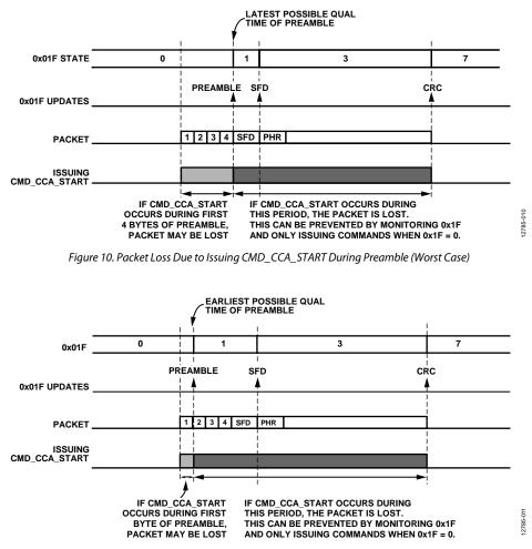
Figure 11. Packet Loss Due to Issuing CMD\_CCA\_START During Preamble (Best Case)
