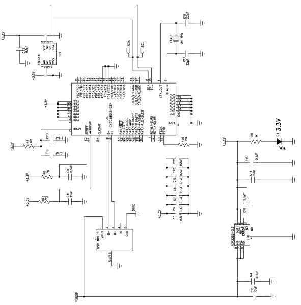
Figure 6. Schematic of USB Controller Circuitry
