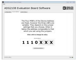
Figure 4. Device Address Tab
