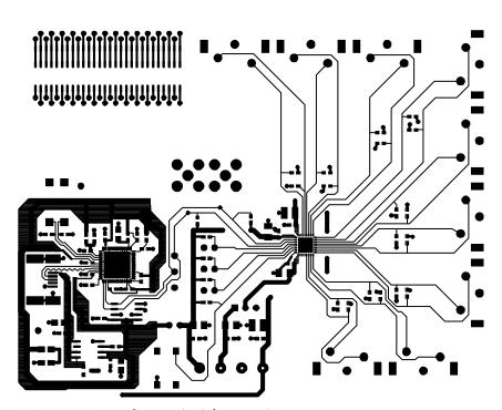
Eval-ADG2108EBZ Rev. 0 - (Component Side View) Component Side
