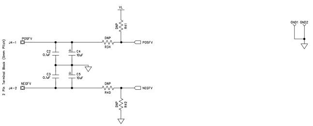
Figure 5. ADG5248F Evaluation Board Schematic (Part 3)
