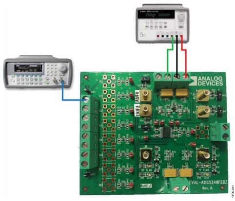
$Figure\ 1. The\ \textit{EVAL-ADG5248FEBZ}\ (on\ the\ Lower\ Right),\ Power\ Supply\ (on\ the\ Top\ Right),\ and\ Signal\ Generator\ (on\ the\ Left)$
