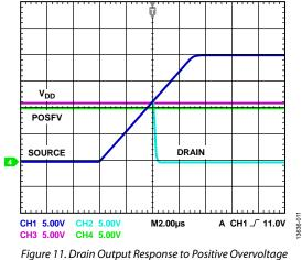
gure 11. Drain Output Response to Positive Overvoltage (Diode from VDD to POSFV)
