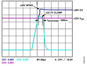
Figure 7. Overshoot During Fault Condition
