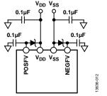
Figure 12. Zener Diode Configured Secondary Supply Rails
