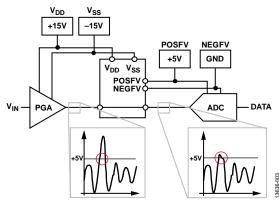
Figure 3. ADG5462F Channel Protector Application Example
