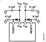
Figure 10. Diodes Configured Secondary Supply Rails
