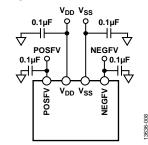
Figure 8. Separate Low Impedance Secondary Supply Rails
