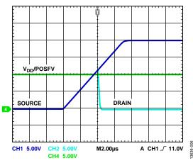
Figure 6. Drain Output Response to Positive Overvoltage (POSFV Tied to VDD)
