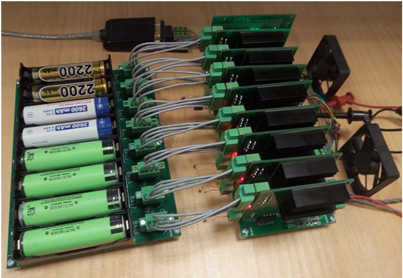
Figure 14. Complete Battery Testing System Connected to Eight Batteries
