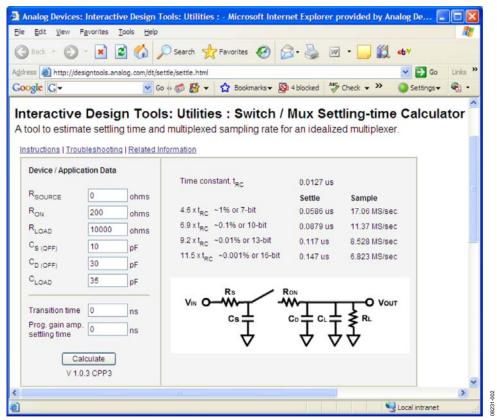
Figure 2. Switch/Multiplexer Calculator Tool
