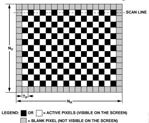
Figure 4. Pixels in a Scanned Image
