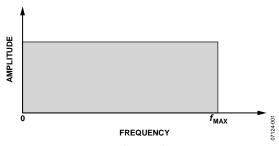
Figure 1. Video Signal Spectrum.
